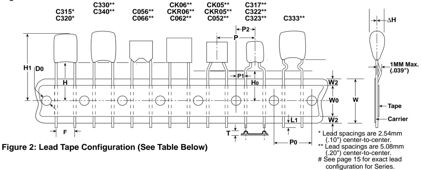
Figure 2: Lead Tape Configuration (See Table Below)
