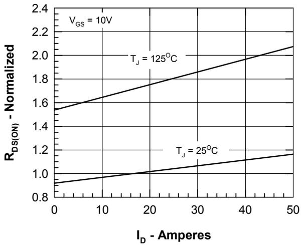
Figure 3.  $R_{DS(on)}$  normalized to 0.5  $I_{D25}$  value vs.  $I_D$
