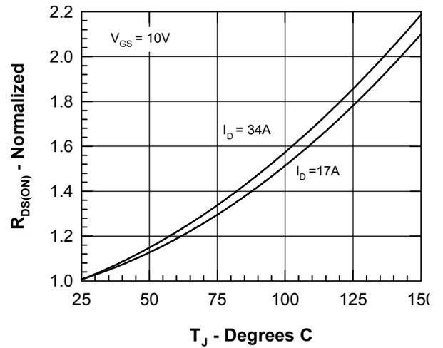
Figure 4.  $R_{DS(on)}$  normalized to 0.5  $I_{D25}$  value vs.  $T_J$
