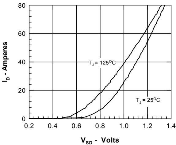
Figure 8. Forward Voltage Drop of the Intrinsic Diode
