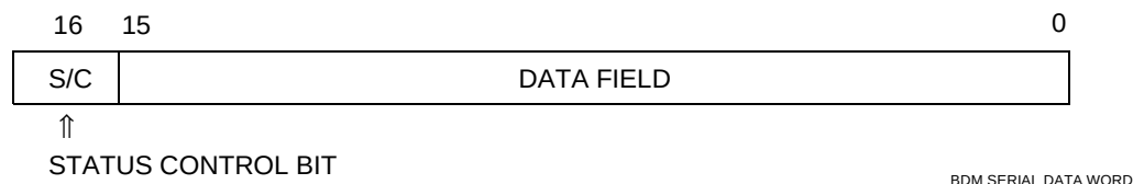
Figure 3-11 BDM Serial Data Word
