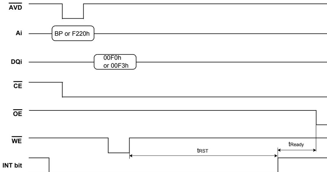
Figure 37. Reset Timing
