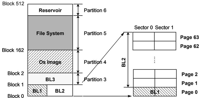
Figure 26. Partition of NAND Flash array
