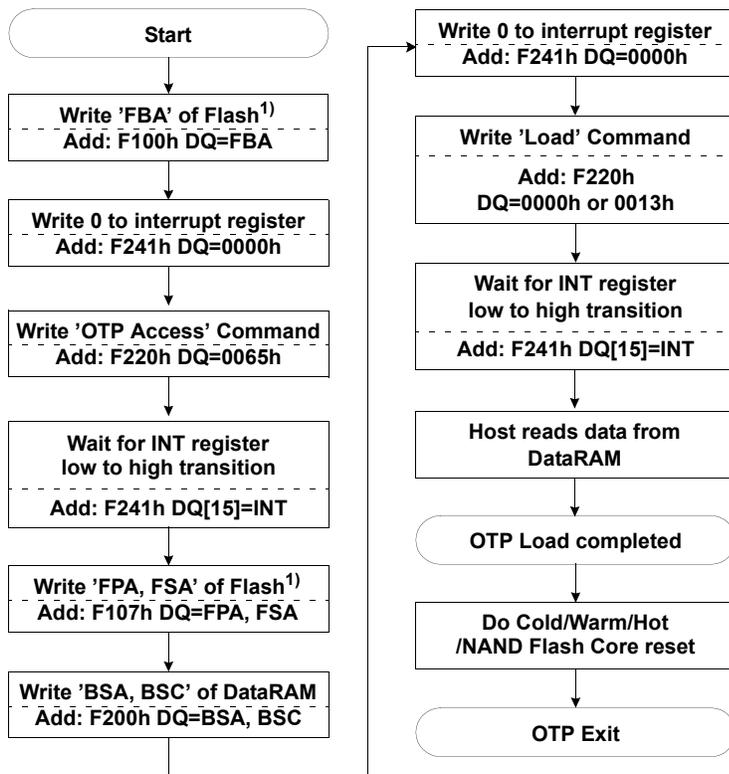
Note 1) FBA(NAND Flash Block Address) could be omitted or any address.
