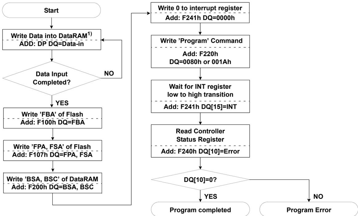
\* : If program operation results in an error, map out the block including the page in error and copy the target data to another block.
