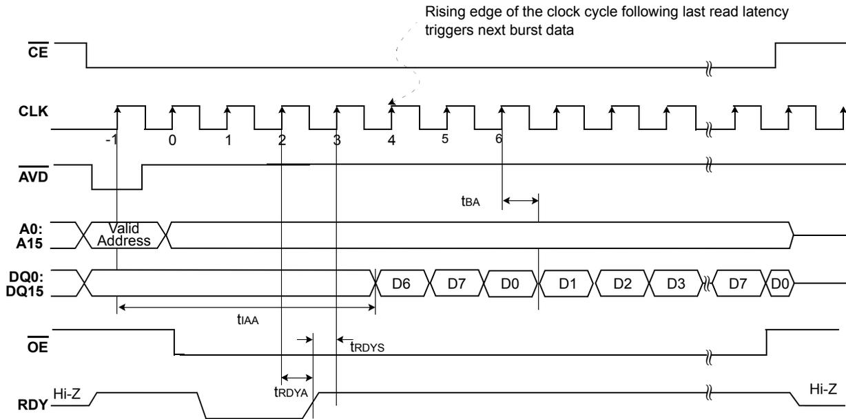
**Figure 13. Example of 4 clock Burst Read Latency**
