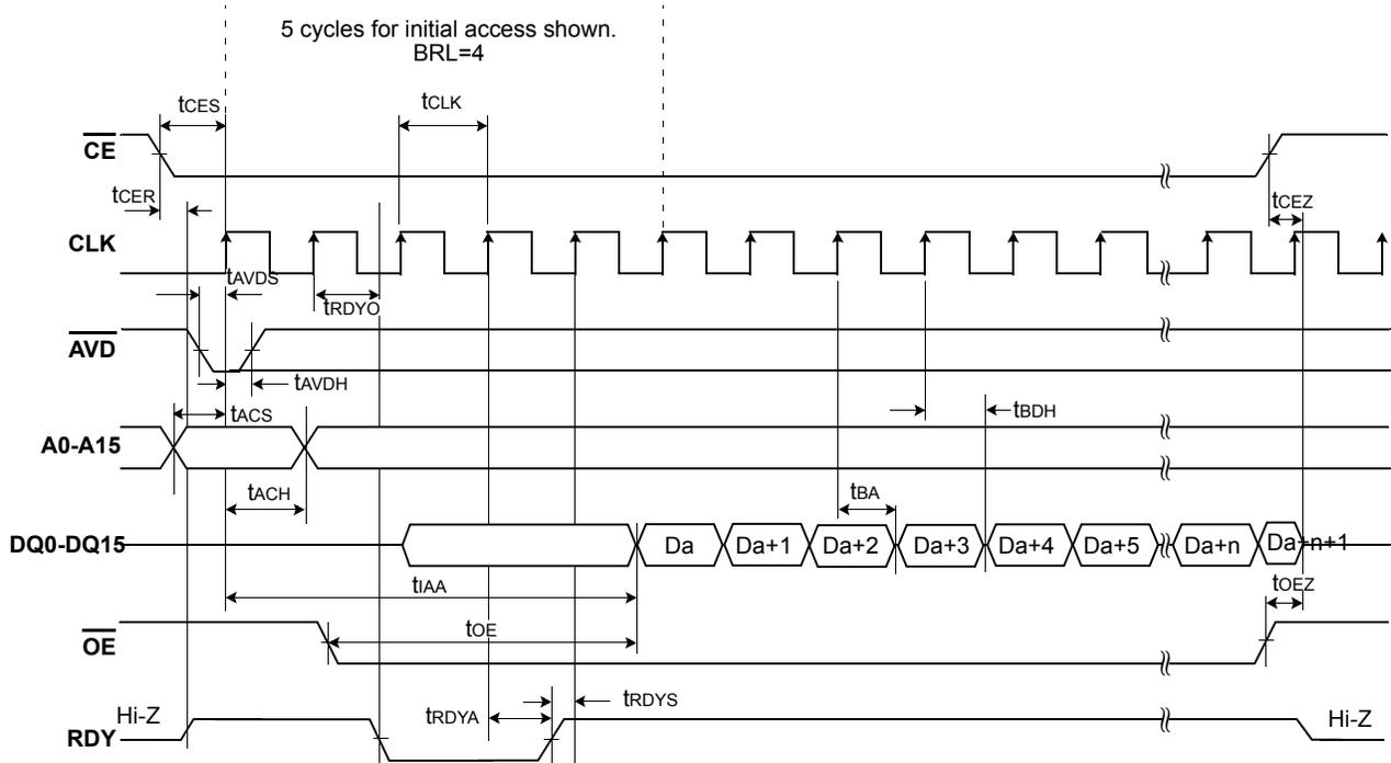
Figure 29. Continuous Linear Burst Mode with Wrap Around
