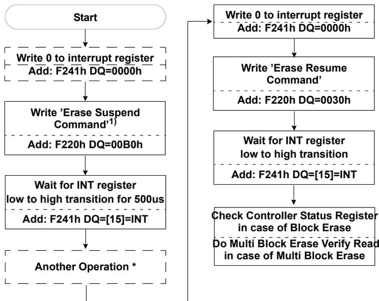
\* Another Operation ; Load, Program Copy-back Program, OTP Access<sup>2)</sup>, Hot Reset, Flash Reset, CMD Reset, Multi Block Erase Verify, Lock, Lock-tight, Unlock
