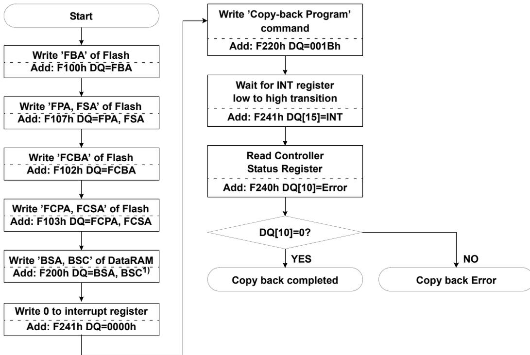
\* : If program operation results in an error, map out the block including the page in error and copy the target data to another block.
