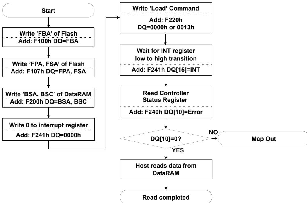
Figure 11. Load operation flow-chart
