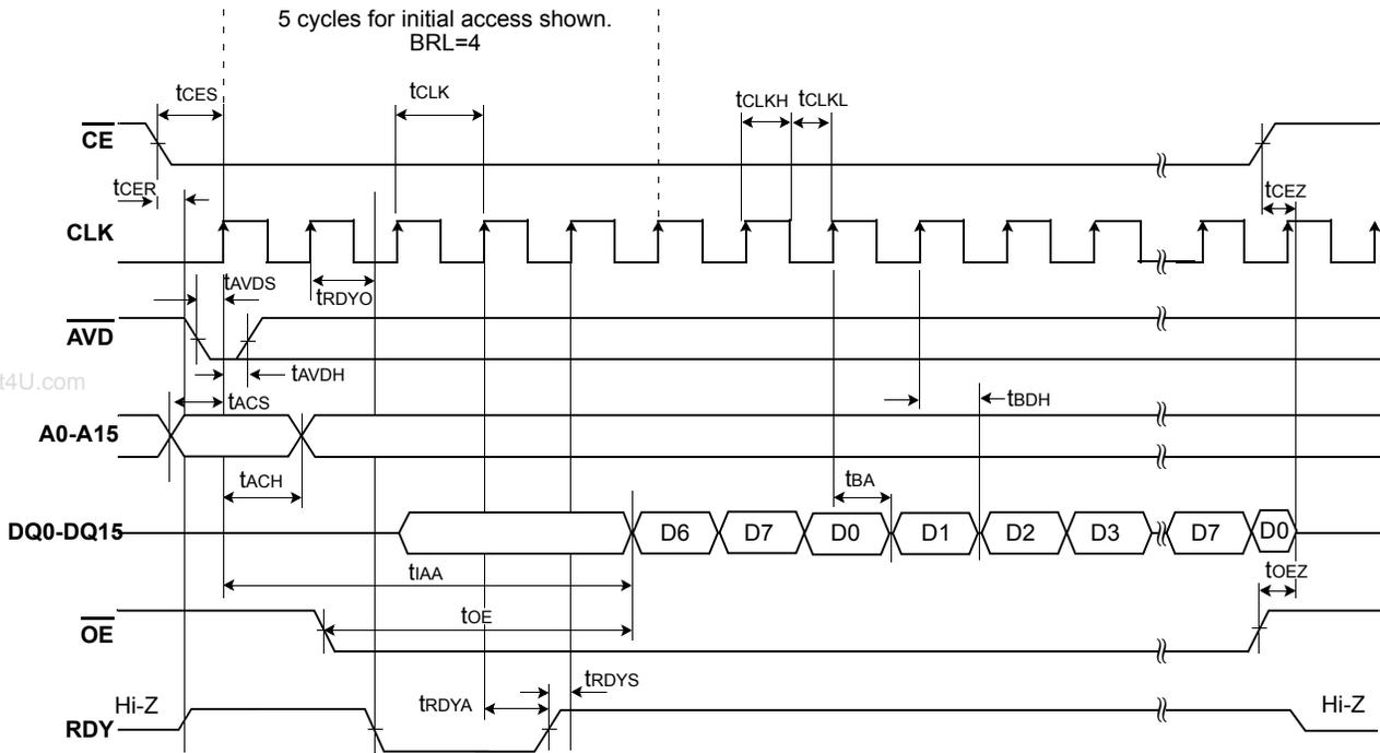
Figure 28. 8 Word Linear Burst Mode with Wrap Around
