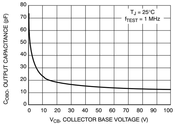
Figure 11. Output Capacitance
