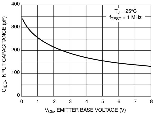
Figure 10. Input Capacitance
