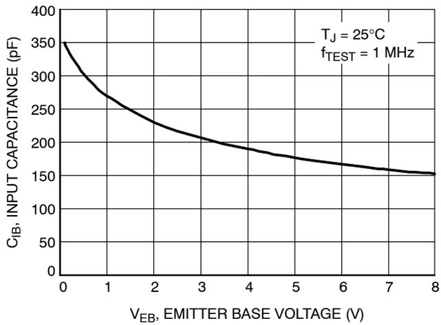
Figure 10. Input Capacitance
