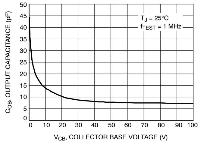
Figure 11. Output Capacitance
