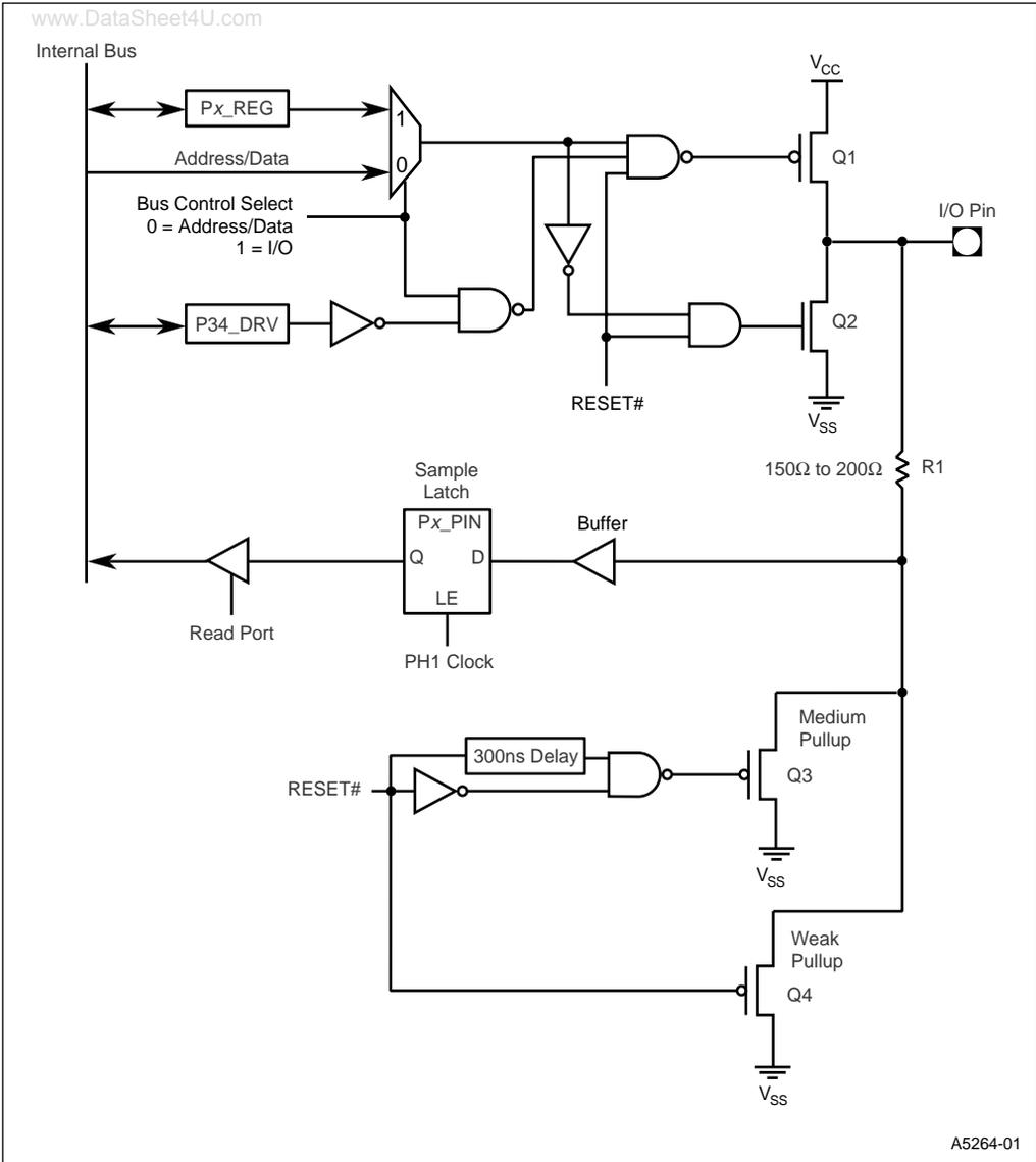
Figure 5-2. Ports 3 and 4 Internal Structure (87C196LA, LB Only)
