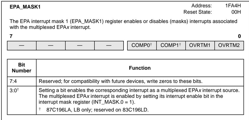
**Figure 7-4. EPA Interrupt Mask 1 (EPA\_MASK1) Register**
