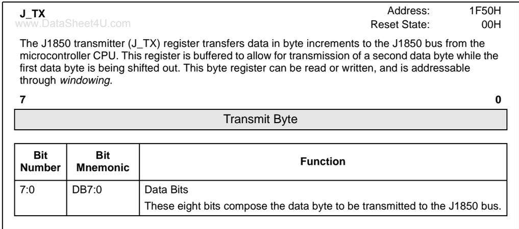
**Figure 8-12. J1850 Transmitter (J\_TX) Register**
