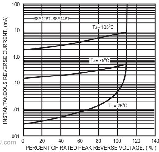
FIG. 3B - TYPICAL REVERSE CHARACTERISTICS
