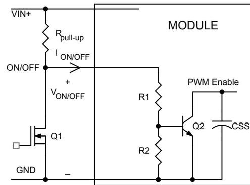
Figure 28. Circuit configuration for using negative logic On/Off.
