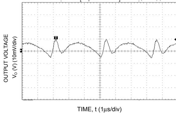
**Figure 8. Typical Output Ripple and Noise**
