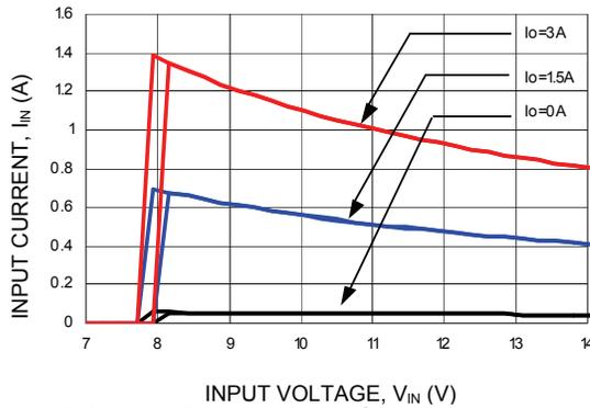
**Figure 7. Input voltage vs. Input Current**
