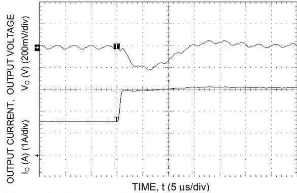
**Figure 10. Transient Response to Dynamic Load Change from 50% to 100% of full load**
