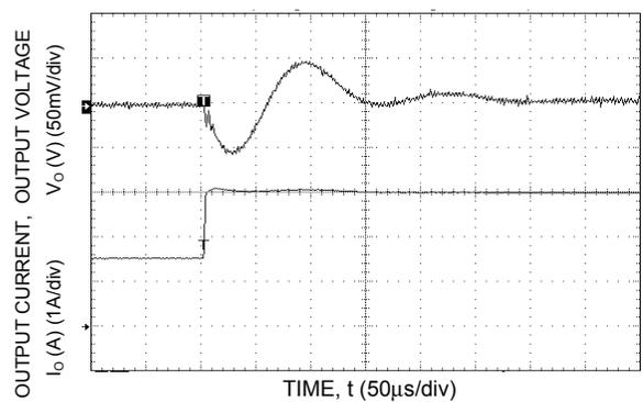
**Figure 12. Transient Response to Dynamic Load Change from 50% to 100% of full load**
