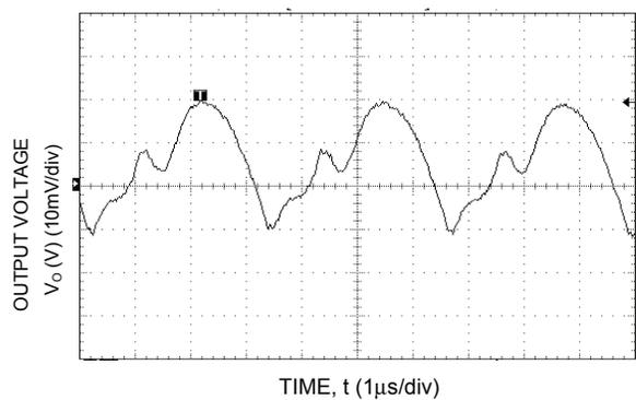
**Figure 9. Typical Output Ripple and Noise**
