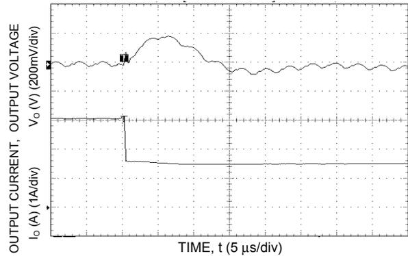
**Figure 11. Transient Response to Dynamic Load Change from 100% to 50% of full load**
