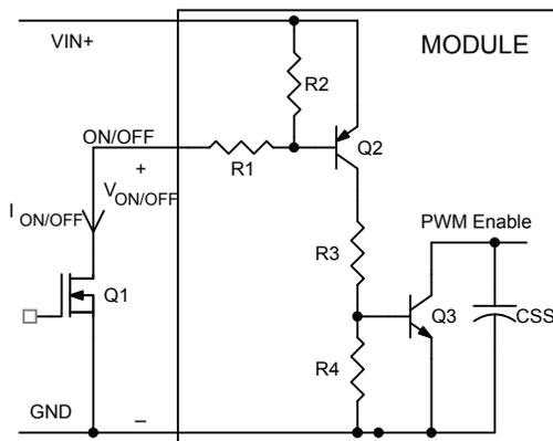
Figure 27. Circuit configuration for using positive logic On/Off.
