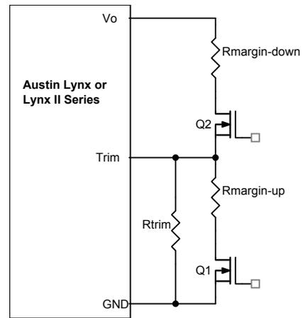
Figure 30. Circuit Configuration for margining Output voltage.
