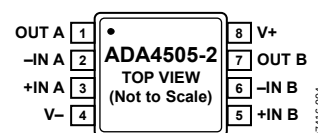
Figure 2. 8-Lead MSOP (RM-8)
