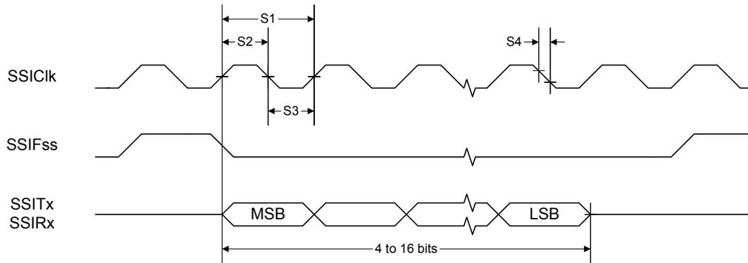
**Figure 19-4. SSI Timing for MICROWIRE Frame Format (FRF=10), Single Transfer**
