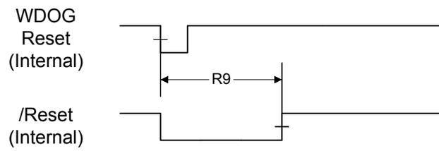
**Figure 19-14. LDO Reset Timing**
