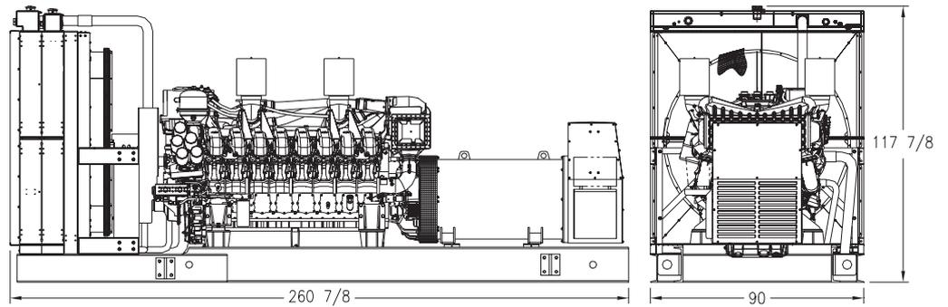
Drawing above for illustration purposes only, based on standard open power 480 volt generator. Lengths may vary with other voltages. Do not use for installation design.
