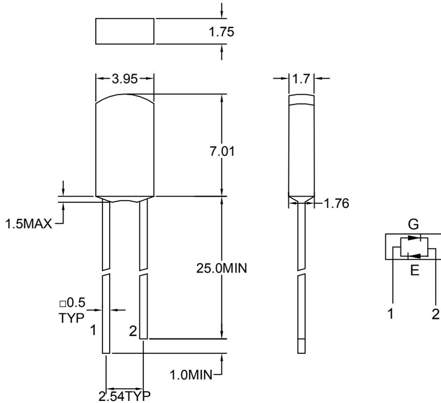
Note : 1.All dimension are in millimeter tolerance is  $\pm 0.25\text{mm}$  unless otherwise noted.
