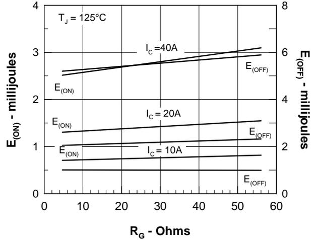
Fig. 8. Dependence of  $E_{ON}$  and  $E_{OFF}$  on  $R_G$ .
