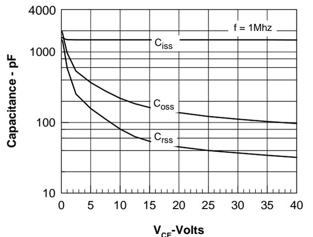
Fig. 6. Capacitance Curves
