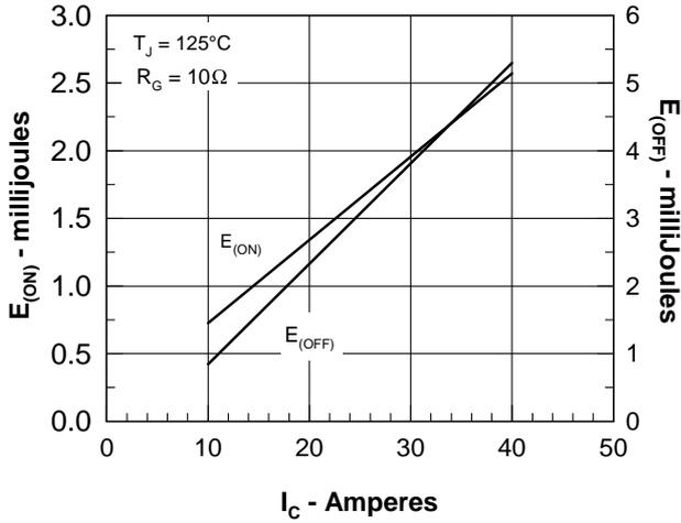
Fig. 7. Dependence of  $E_{ON}$  and  $E_{OFF}$  on  $I_C$ .
