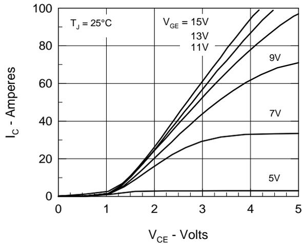
Fig. 1. Output Characteristics
