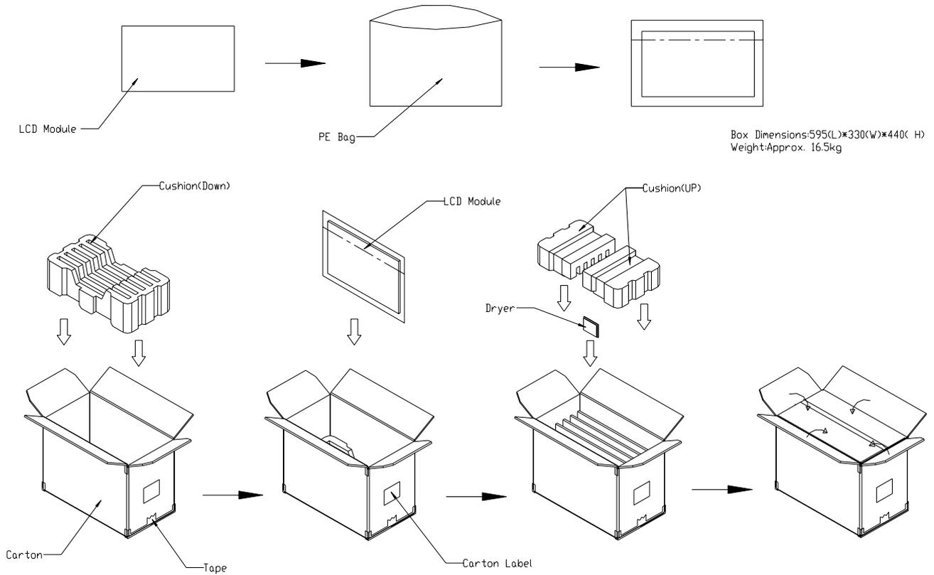
**Figure. 8-1 Packing method**
