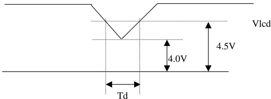
Dip condition:  **$4.0\text{ V} \leq V_{lcd} \leq 4.5\text{ V}, T_d \leq 20\text{ ms}$**
