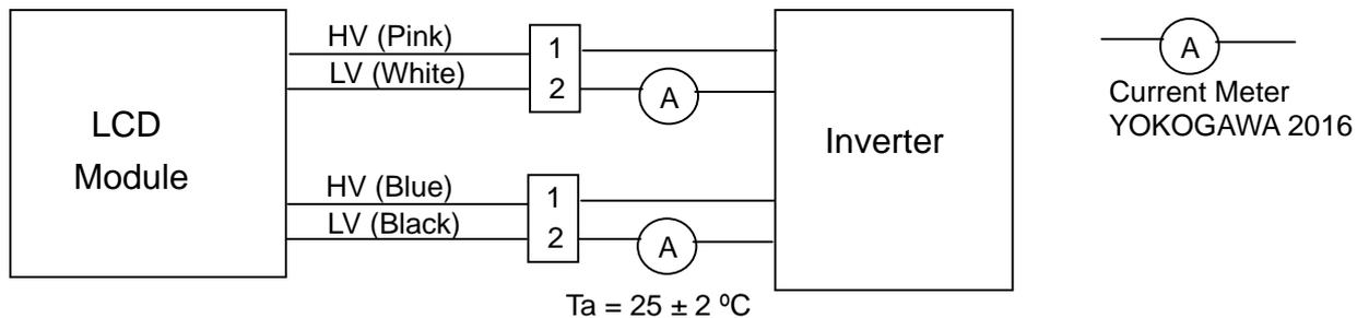
Note (2) The voltage that must be larger than  $V_S$  should be applied to the lamp for more than 1 second after startup. Otherwise, the lamp may not be turned on normally.
