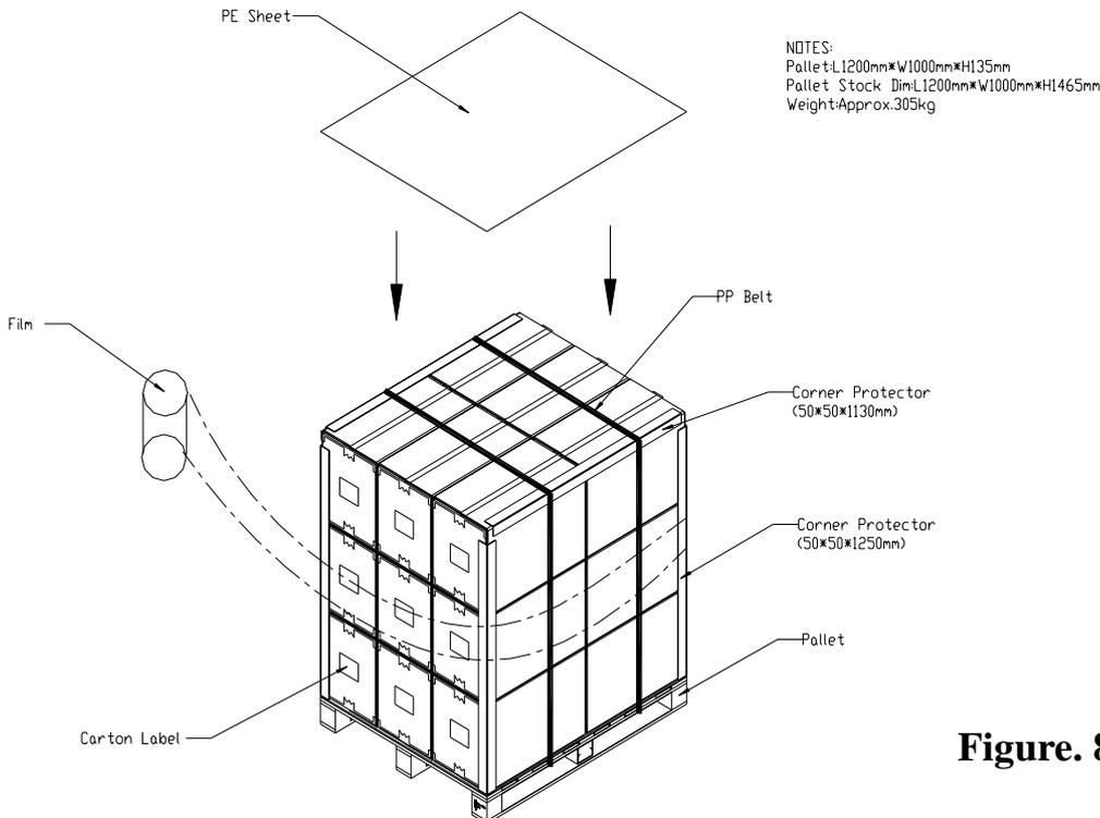
**Figure. 8-3 Packing method**
