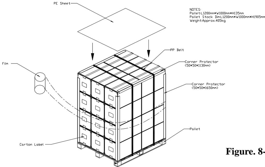
**Figure. 8-2 Packing method**
