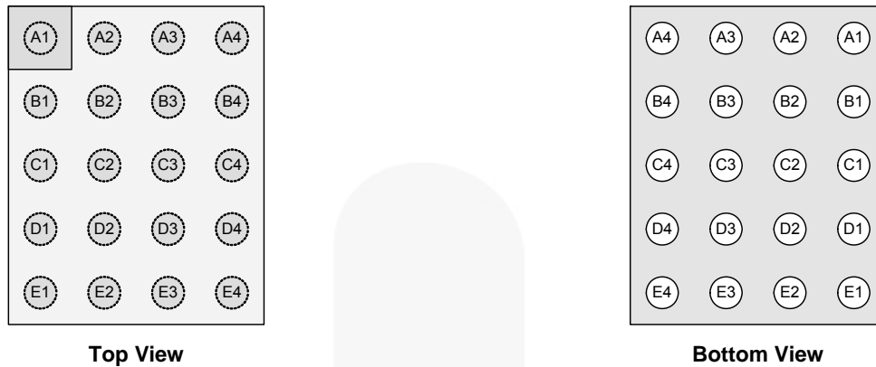
Figure 4. WLCSP-20 Pin Assignments
