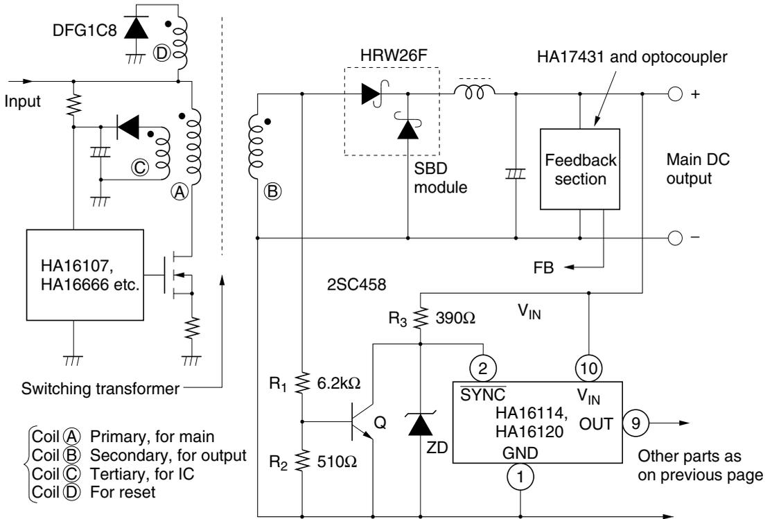
This circuit illustrates the combination of the HA16114/120 with a forward AC/DC converter. The HA16114/120 synchronizes with the falling edge of the external sync signal, so with a forward transformer, the sync pulses must be inverted. In the diagram, this is done by an external circuit consisting of the following components:
