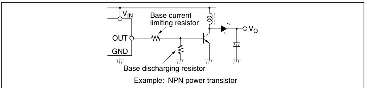
**Figure 4.3 Driving a Bipolar Power Transistor**
