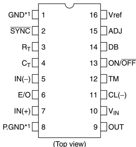
Note: 1. Pin 1 (GND) and Pin 8 (P.GND) must be connected each other with external wire.
