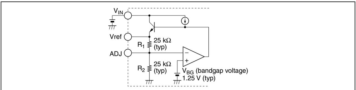
Figure 5.2 Simplified Diagram of Voltage Reference Circuit
