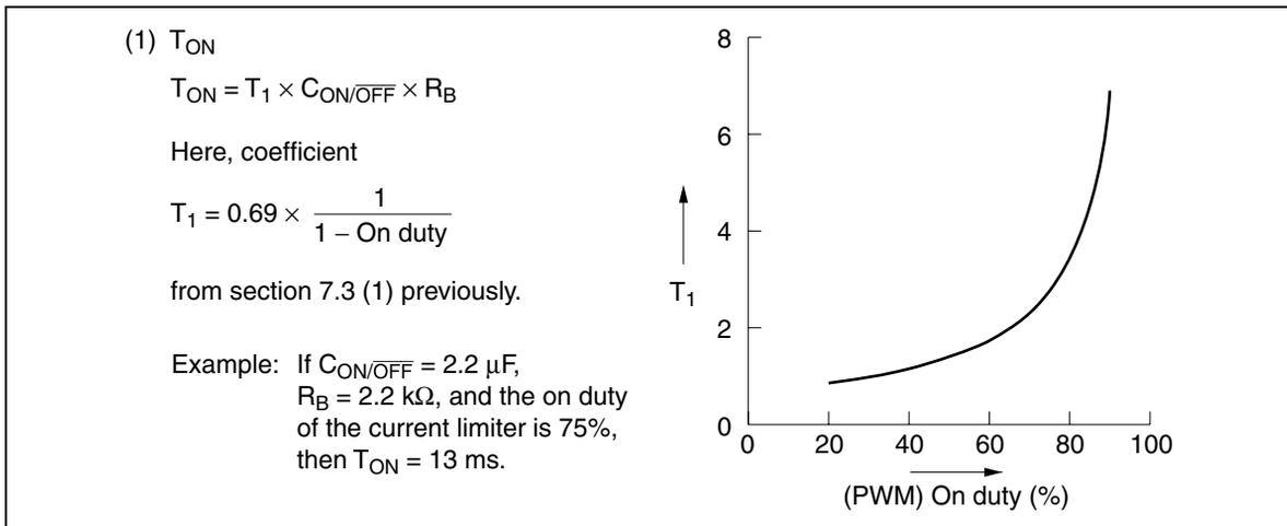
Figure 7.4 Examples of Intermittent Mode Timing (1)
