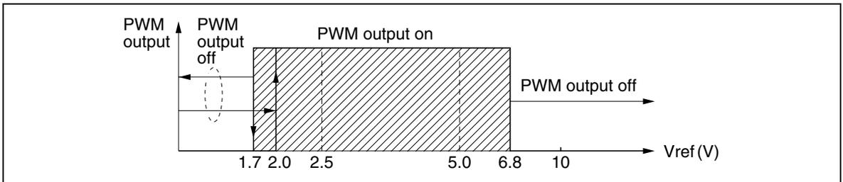
**Figure 5.4 Vref Undervoltage Lockout and Overvoltage Protection**
