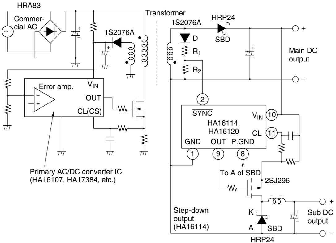
This is one example of a circuit that uses the features of the HA16114/120 by operating in synchronization with a flyback AC/DC converter. Note the following design points concerning the circuit from the secondary side of the transformer to the  $\overline{\text{SYNC}}$  pin of the HA16114/120.
