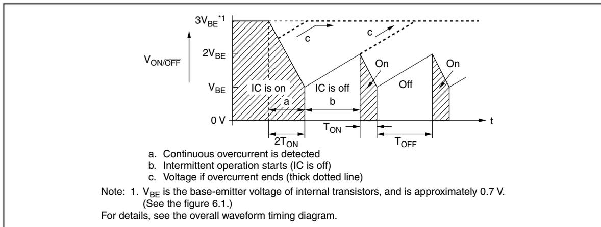
Figure 7.2 Intermittent Mode Timing Diagram ( $V_{ON/OFF}$  only)
