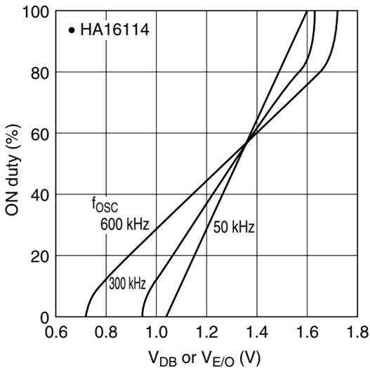
Note: The on-duty of the HA16114 is the proportion of one cycle during which output is low.
