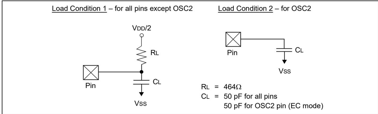
**TABLE 30-16: CAPACITIVE LOADING REQUIREMENTS ON OUTPUT PINS**
