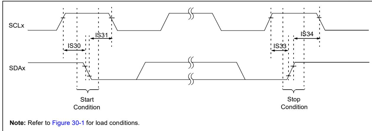
**FIGURE 30-17: I2Cx BUS DATA TIMING CHARACTERISTICS (SLAVE MODE)**
