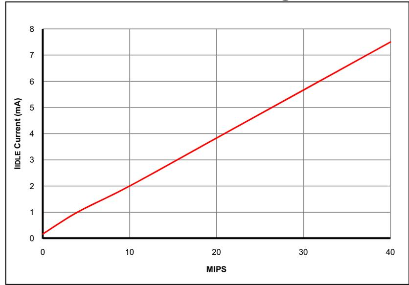
**FIGURE 32-4: TYPICAL I<sub>DD</sub> CURRENT @ V<sub>DD</sub> = 3.3V**
