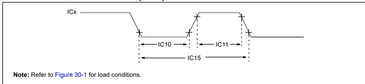
**TABLE 30-25: INPUT CAPTURE MODULE TIMING REQUIREMENTS**
