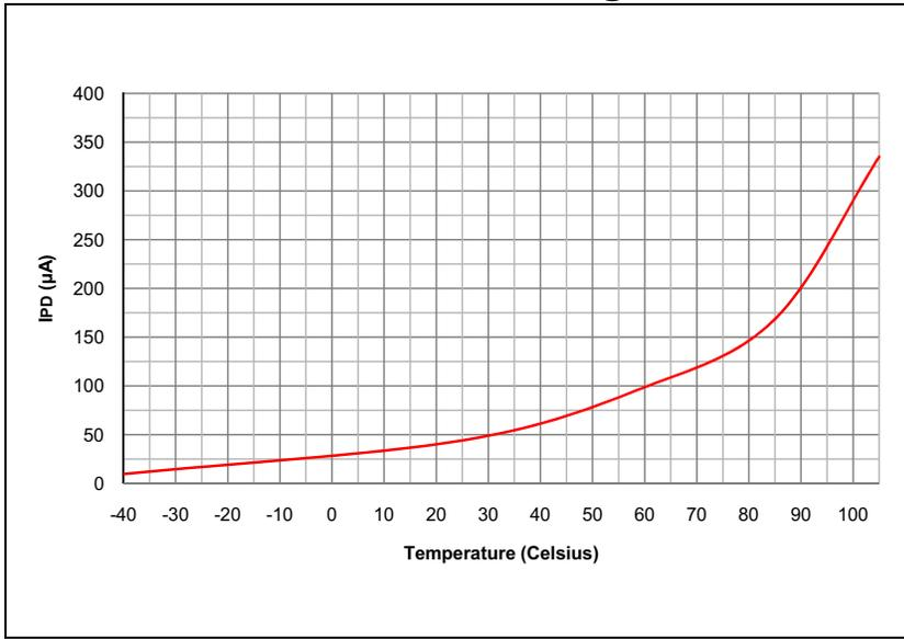
**FIGURE 32-5: TYPICAL I<sub>IDLE</sub> CURRENT @ V<sub>DD</sub> = 3.3V**
