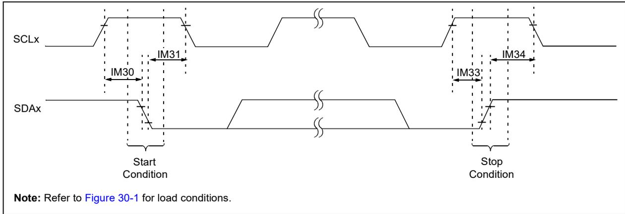
**FIGURE 30-15: I2Cx BUS DATA TIMING CHARACTERISTICS (MASTER MODE)**
