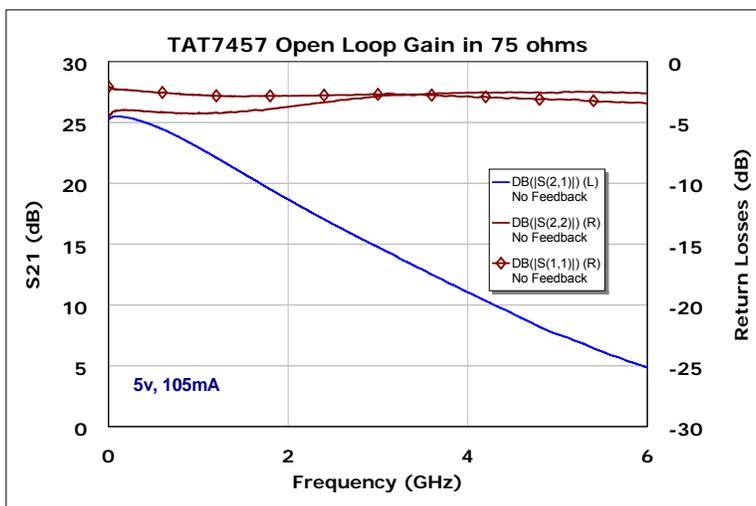
There are no on-chip capacitors that limit the low frequency response, enabling the TAT7457 frequency response to extend to DC. The open loop gain (no external feedback) and high frequency gain performance is shown in the plot to the left.
