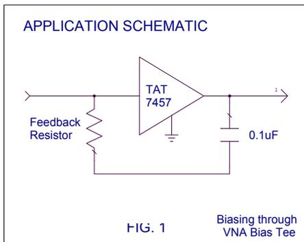
Customers may set the gain and return loss of their amplifier by selecting an appropriate external feedback resistor.
