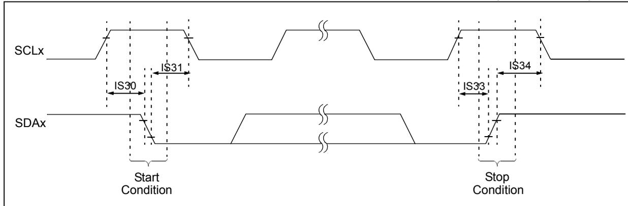
**FIGURE 25-20: I2Cx BUS DATA TIMING CHARACTERISTICS (SLAVE MODE)**
