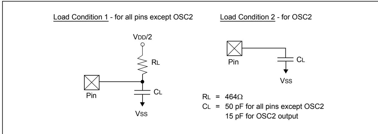
**TABLE 25-15: CAPACITIVE LOADING REQUIREMENTS ON OUTPUT PINS**
