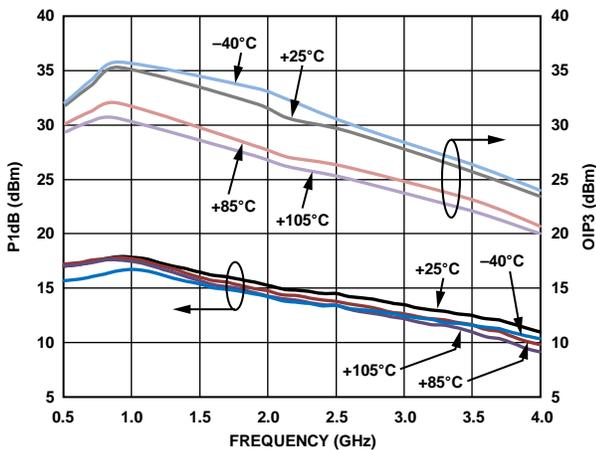
Figure 5. P1dB and OIP3 vs. Frequency and Temperature
