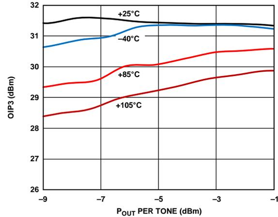
Figure 37. OIP3 vs. P<sub>OUT</sub> at 30 MHz
