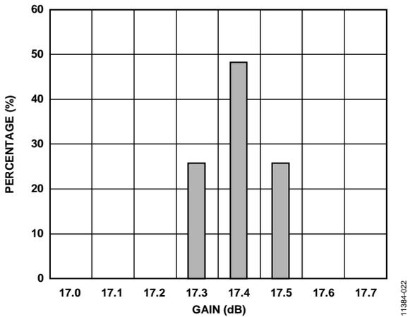
Figure 22. Gain Distribution at 900 MHz
