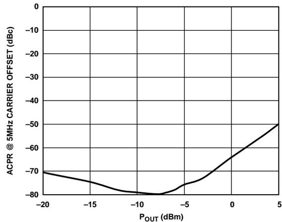
Figure 38. ACPR vs. P<sub>OUT</sub>, Single W-CDMA Carrier (Test Model 1-64) at 2140 MHz
