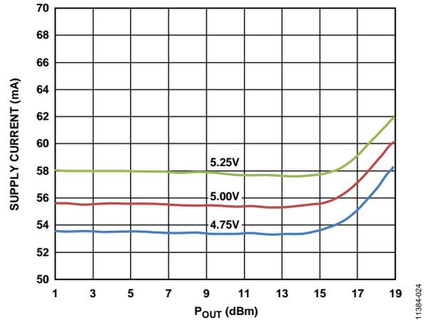
Figure 24. Supply Current vs. POUT at 900 MHz
