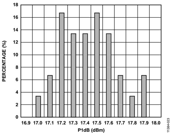
Figure 23. P1dB Distribution at 900 MHz
