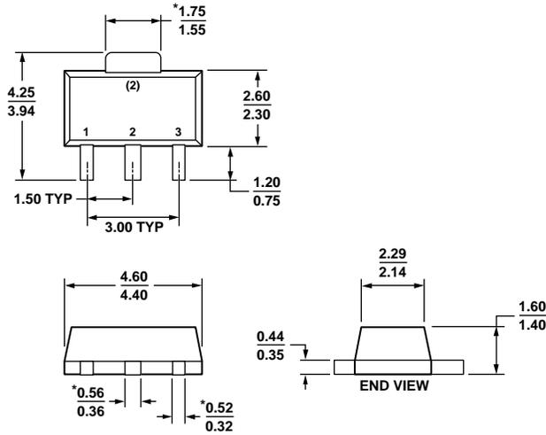
\*COMPLIANT TO JEDEC STANDARDS TO-243 WITH THE EXCEPTION OF DIMENSIONS INDICATED BY AN ASTERISK.
