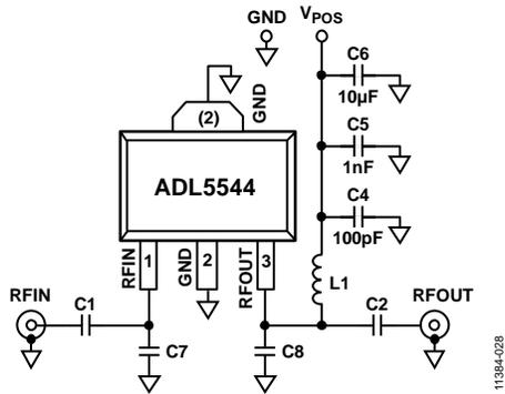
Figure 28. Basic Connections
