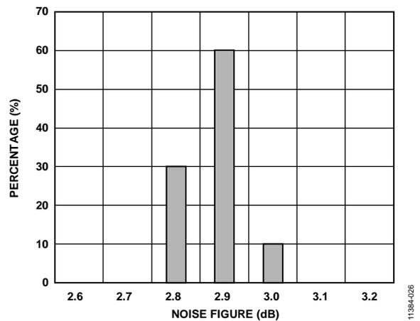
Figure 26. Noise Figure Distribution at 900 MHz
