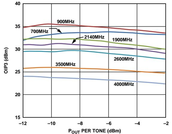
Figure 6. OIP3 vs. Output Power ( $P_{OUT}$ ) and Frequency
