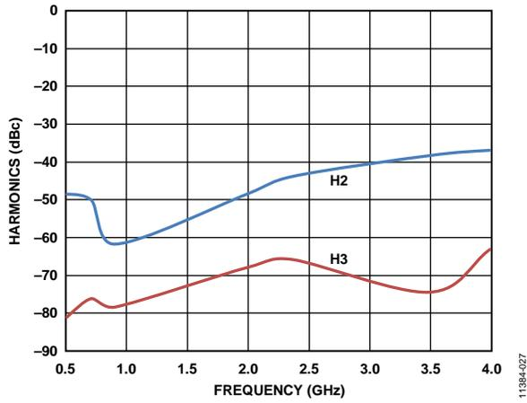
Figure 27. Single-Tone Harmonics vs. Frequency,  $P_{OUT} = 0 \text{ dBm}$
