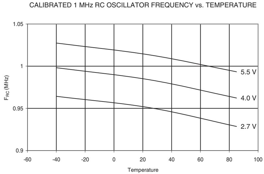
**Figure 28-47.** Calibrated 1 MHz RC Oscillator Frequency vs.  $V_{CC}$
