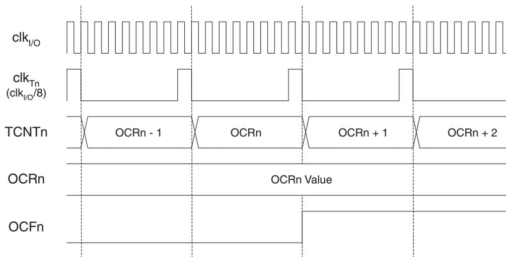
Figure 17-11 shows the setting of OCF2 and the clearing of TCNT2 in CTC mode.
