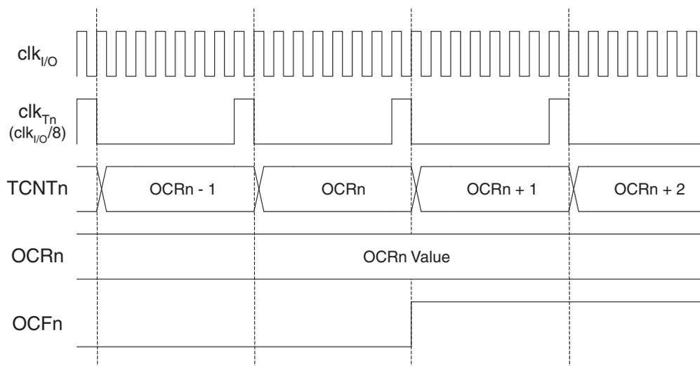
Figure 14-11 shows the setting of OCF0 and the clearing of TCNT0 in CTC mode.
