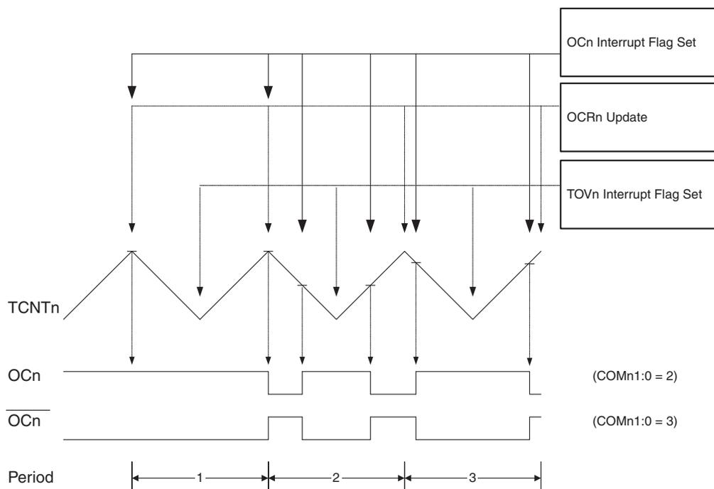
The Timer/Counter Overflow Flag (TOV0) is set each time the counter reaches BOTTOM. The Interrupt Flag can be used to generate an interrupt each time the counter reaches the BOTTOM value.
