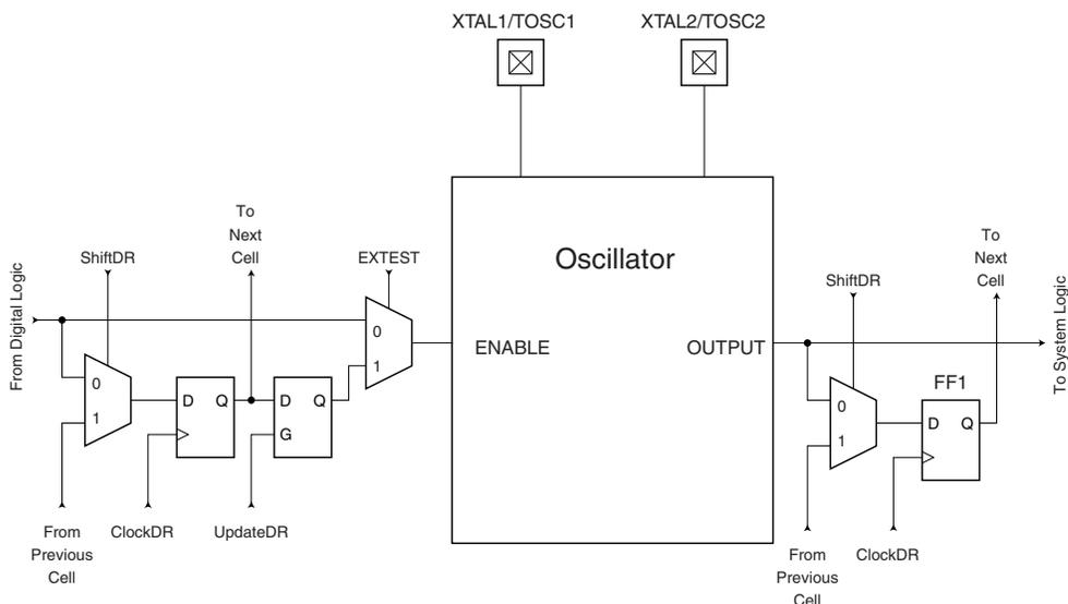
Table 24-4 summarizes the scan registers for the external clock pin XTAL1, Oscillators with XTAL1/XTAL2 connections as well as 32 kHz Timer Oscillator.
