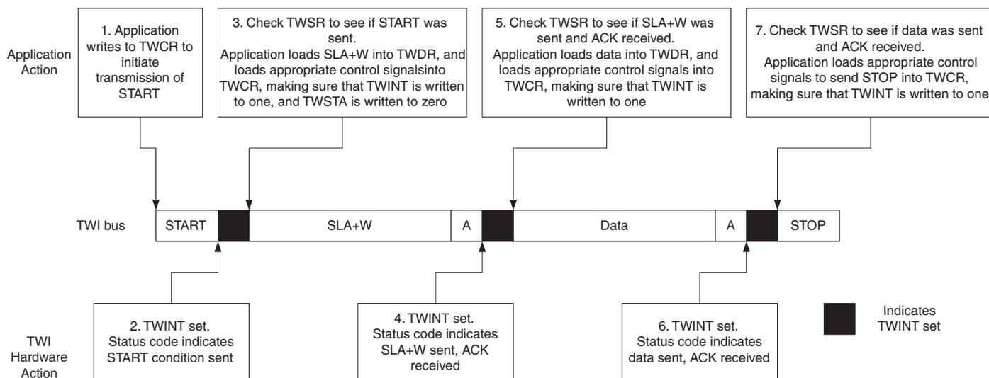
1. The first step in a TWI transmission is to transmit a START condition. This is done by writing a specific value into TWCR, instructing the TWI hardware to transmit a START condition. Which value to write is described later on. However, it is important that the TWINT bit is set in the value written. Writing a one to TWINT clears the flag. The TWI will not start any operation as long as the TWINT bit in TWCR is set. Immediately after
