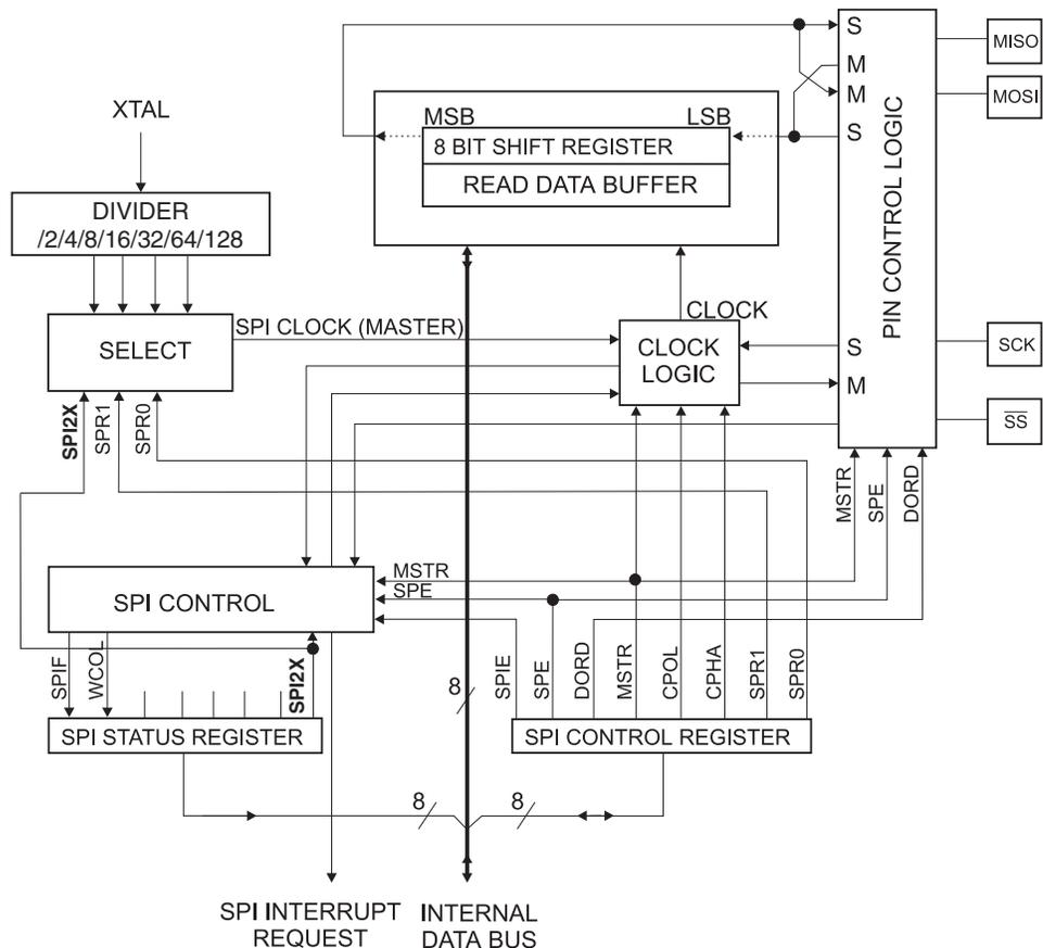
Note: 1. Refer to [Figure 1-1 on page 2](#), and [Table 12-6 on page 57](#) for SPI pin placement.
