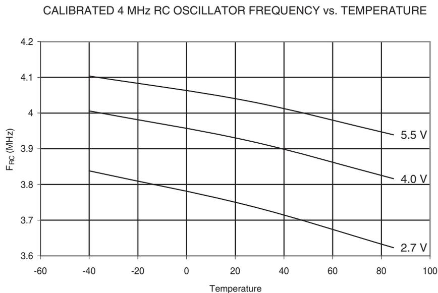
**Figure 28-41.** Calibrated 4 MHz RC Oscillator Frequency vs.  $V_{CC}$
