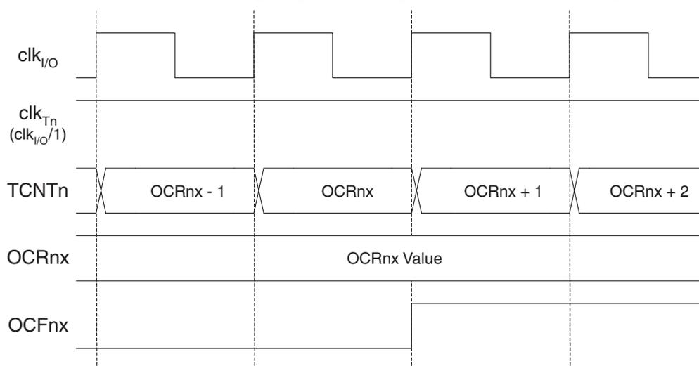
[Figure 16-11](#) shows the same timing data, but with the prescaler enabled.
