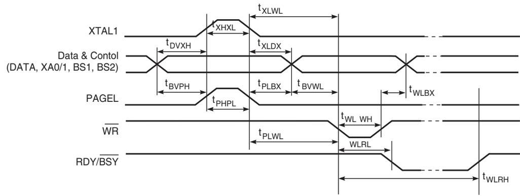
**Figure 27-9. Parallel Programming Timing, Loading Sequence with Timing Requirements<sup>(1)</sup>**
