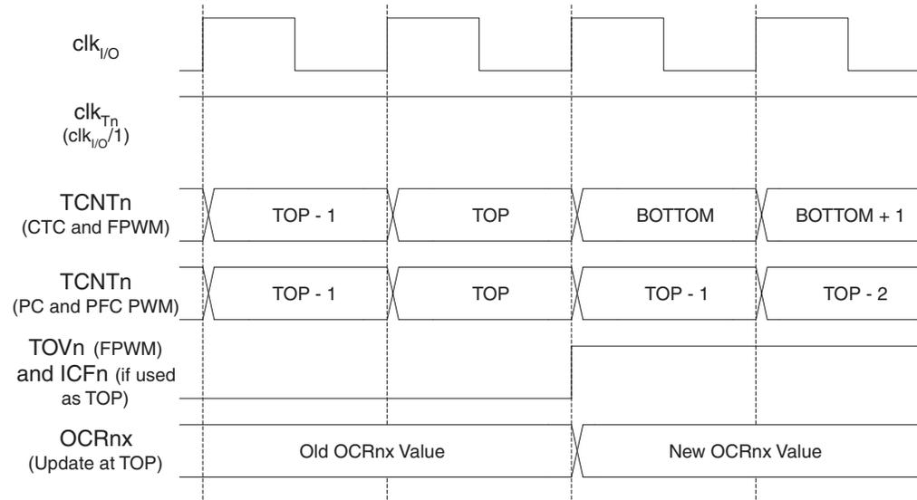
Figure 16-13 shows the same timing data, but with the prescaler enabled.
