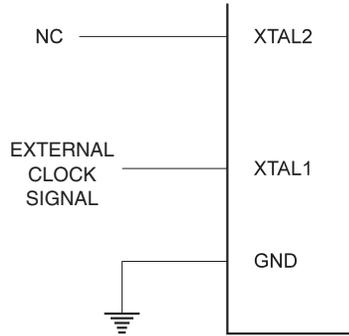
When this clock source is selected, start-up times are determined by the SUT Fuses as shown in [Table 8-10](#).
