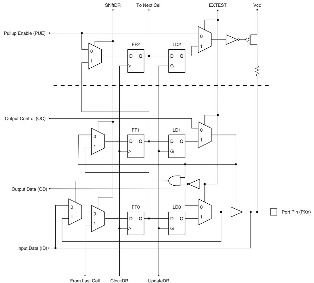
**Figure 24-4. General Port Pin Schematic Diagram<sup>(1)</sup>**
