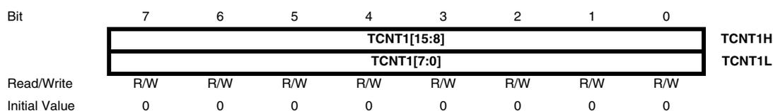
The two *Timer/Counter* I/O locations (TCNT1H and TCNT1L, combined TCNT1) give direct access, both for read and for write operations, to the Timer/Counter unit 16-bit counter. To
