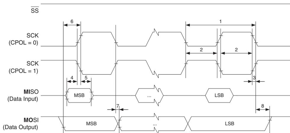
**Figure 27-7. SPI Interface Timing Requirements (Slave Mode)**
