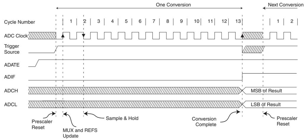
**Figure 22-7. ADC Timing Diagram, Free Running Conversion**
