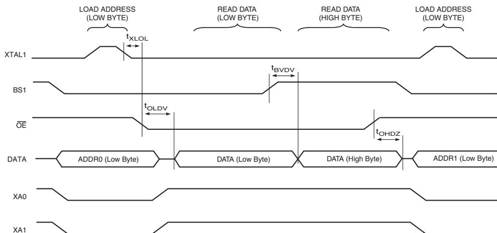
Note: 1. The timing requirements shown in Figure 27-8 (i.e.,  $t_{DVXH}$ ,  $t_{XHXL}$ , and  $t_{XLDX}$ ) also apply to reading operation.
