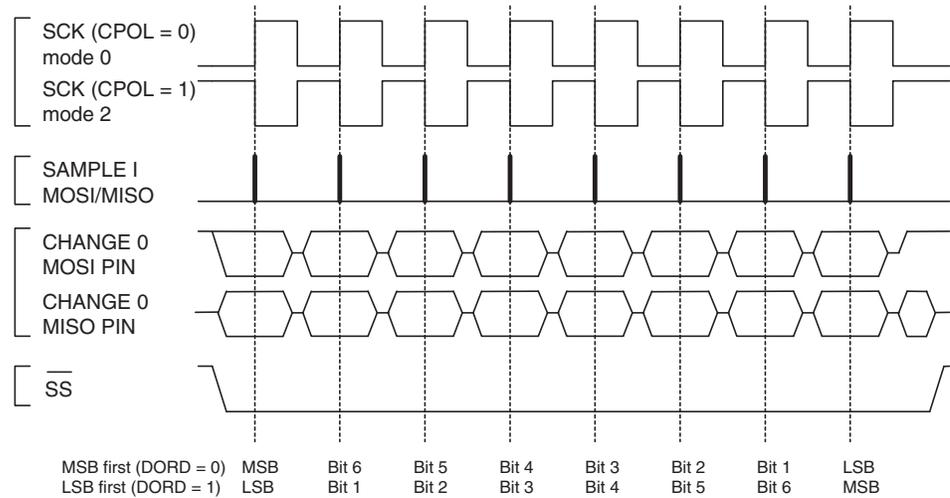
**Figure 18-3. SPI Transfer Format with CPHA = 1**
