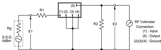
$R_g + R_1 = R_2 = \text{Input/Output Impedance}$
