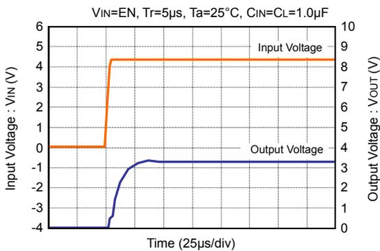
**TYPICAL CHARACTERISTICS – Input Rise Time ( $I_{OUT}=30mA$ )**
