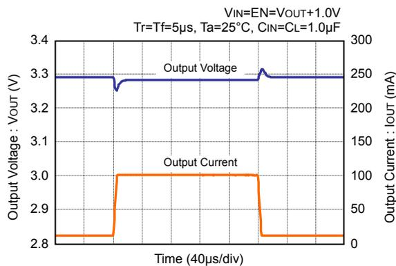
**TYPICAL CHARACTERISTICS – Input Transient Response ( $I_{OUT}=1mA$ )**
