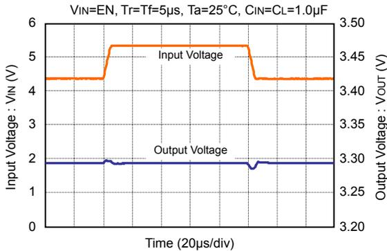
**TYPICAL CHARACTERISTICS – Input Transient Response ( $I_{OUT}=100mA$ )**
