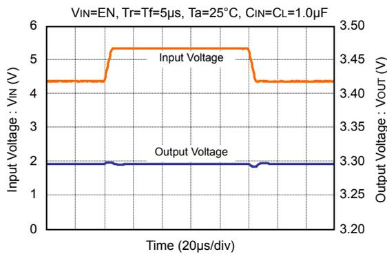
**TYPICAL CHARACTERISTICS – Input Transient Response ( $I_{OUT}=30mA$ )**
