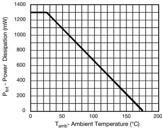
Fig. 1 - Admissible Power Dissipation vs. Ambient Temperature
