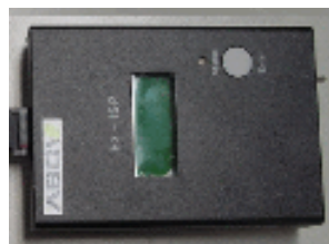
Figure 1-4 Ez-ISP (VDD supplied Standalone type ISP)
