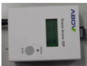
Figure 1-3 StandAlone ISP (VDD power is not supplied)
