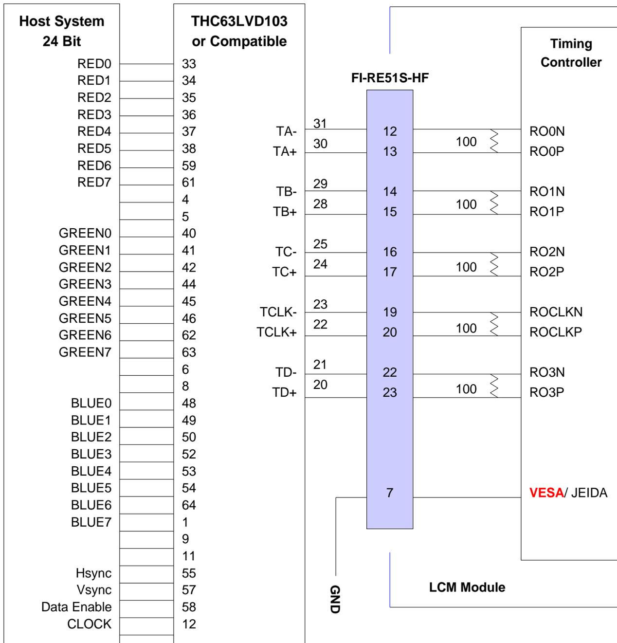
Note: 1. The LCD module uses a 100 Ohm[ ] resistor between positive and negative lines of each receiver input.
