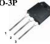
1.Gate 2. Drain 3. Source
