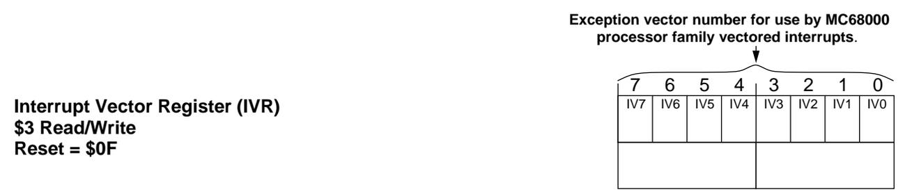
**Figure B-21** Interrupt Vector Register (IVR)
