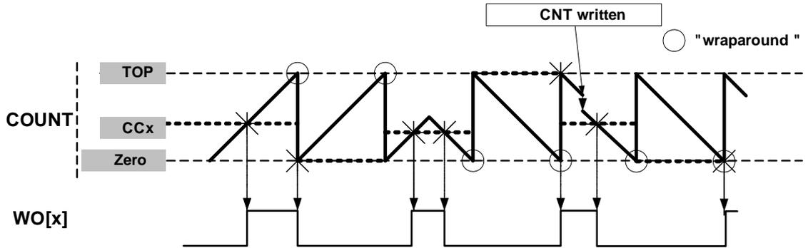
When MFRQ is used, the value in CC0 will be used as the top value and WO[0] will toggle on every overflow/underflow.
