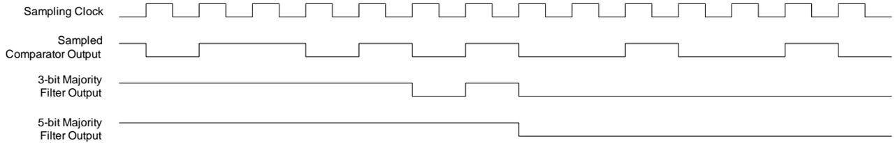
**Figure 29-7. Single-Shot Filtering**
