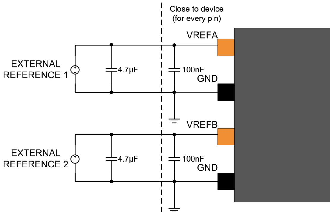
Figure 34-3. External Analog Reference Schematic With One Reference
