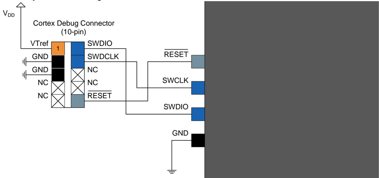
For debuggers/programmers that support the 10-way ARM debug interface should be connected as shown in [Figure 1-10](#) with details described in [Table 1-9](#).
