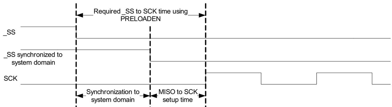
Only one data character written to DATA will be preloaded into the shift register while the synchronized `_SS` signal (see Figure 25-4) is high. The next character written to DATA before `_SS` is pulled low will be stored in DATA until transfer begins. If the shift register is not preloaded, the current contents of the shift register will be shifted out.
