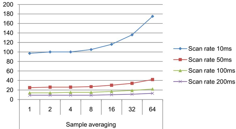
**Figure 32-9. Power consumption [ $\mu$ A].**
