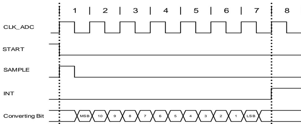
**Figure 28-4. ADC Timing for One Conversion in Differential Mode without Gain, but with Increased Sampling Time**
