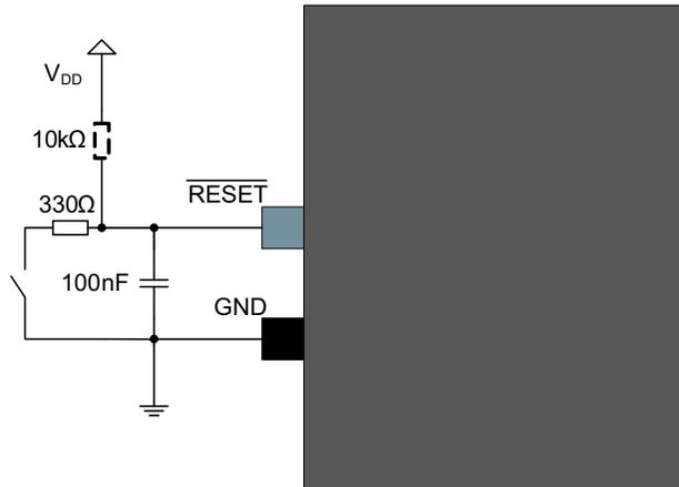
A pull-up resistor makes sure that the reset does not go low unintended causing a device reset. An additional resistor has been added in series with the switch to safely discharge the filtering capacitor, i.e. preventing a current surge when shorting the filtering capacitor which again causes a noise spike that can have a negative effect on the system.
