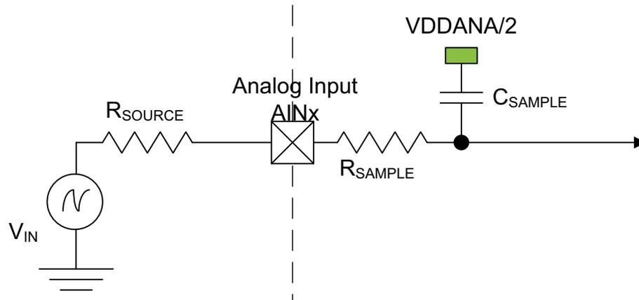
To achieve  $n$  bits of accuracy, the  $C_{SAMPLE}$  capacitor must be charged at least to a voltage of
