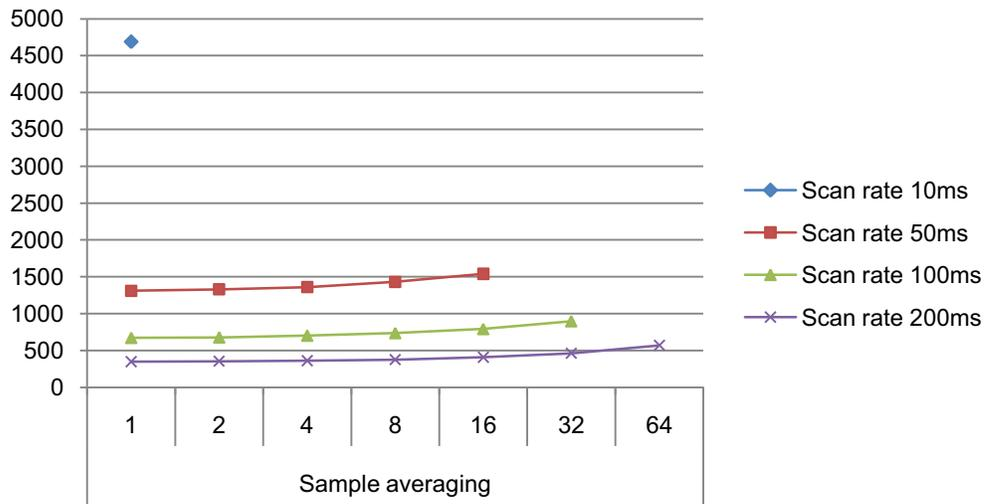
**Figure 32-12. Power consumption [ $\mu$ A].**
