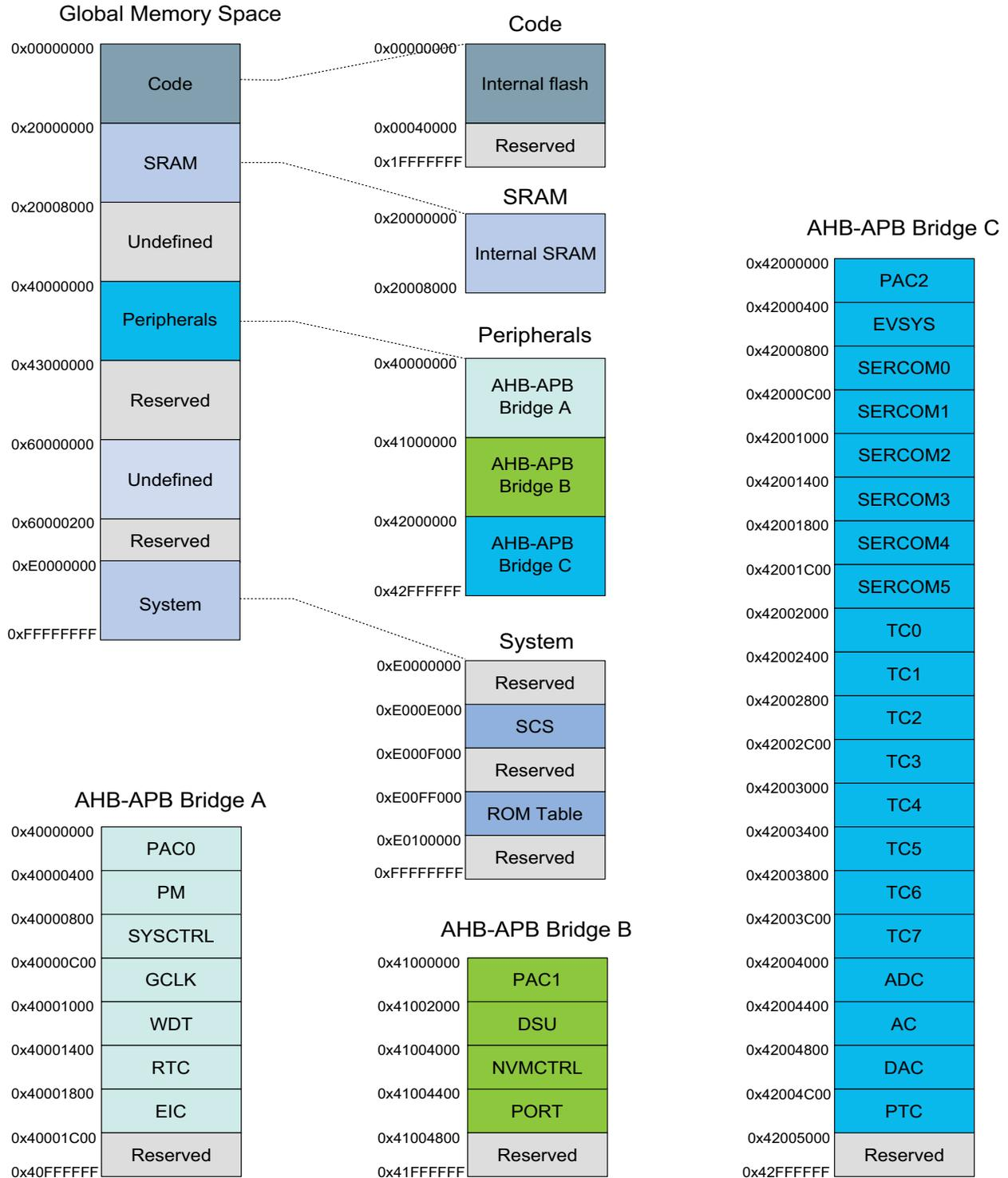
This figure represents the full configuration of the Atmel® SAM D20 with maximum flash and SRAM capabilities and a full set of peripherals. Refer to the “[Configuration Summary](#)” on page 3 for details.
