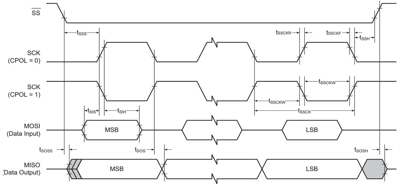
**Table 32-44. SPI timing characteristics and requirements<sup>(1)</sup>**
