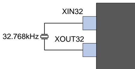
Crystals specifying load capacitance ( $C_L$ ) higher than 12.5pF, require external capacitors applied as described in [Figure 34-8](#).
