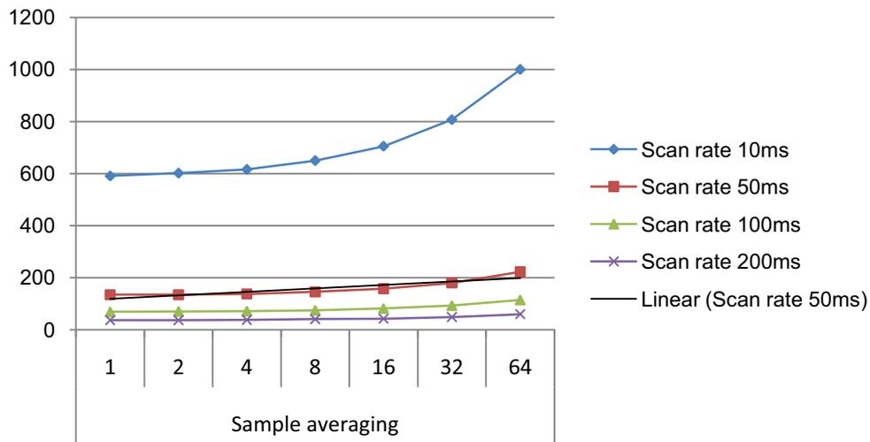
**Figure 32-10. Power consumption [ $\mu$ A].**
