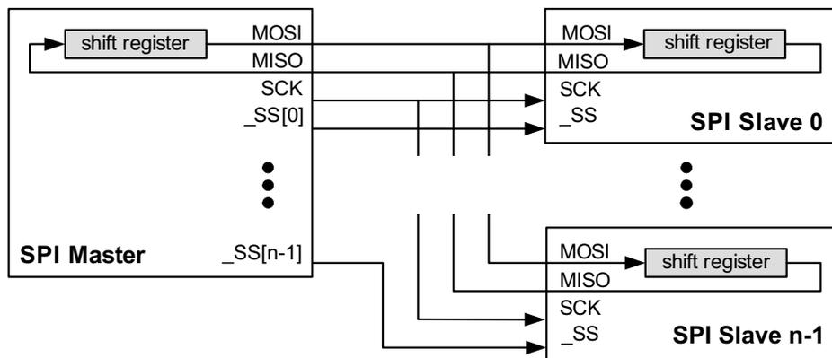
An alternate configuration is shown in [Figure 25-6](#). In this configuration, all n attached slaves are connected in series. A common \_SS line is provided to all slaves, enabling them simultaneously. The master must shift n characters for a complete transaction.
