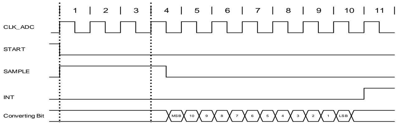
**Figure 28-5. ADC Timing for Free Running in Differential Mode without Gain**
