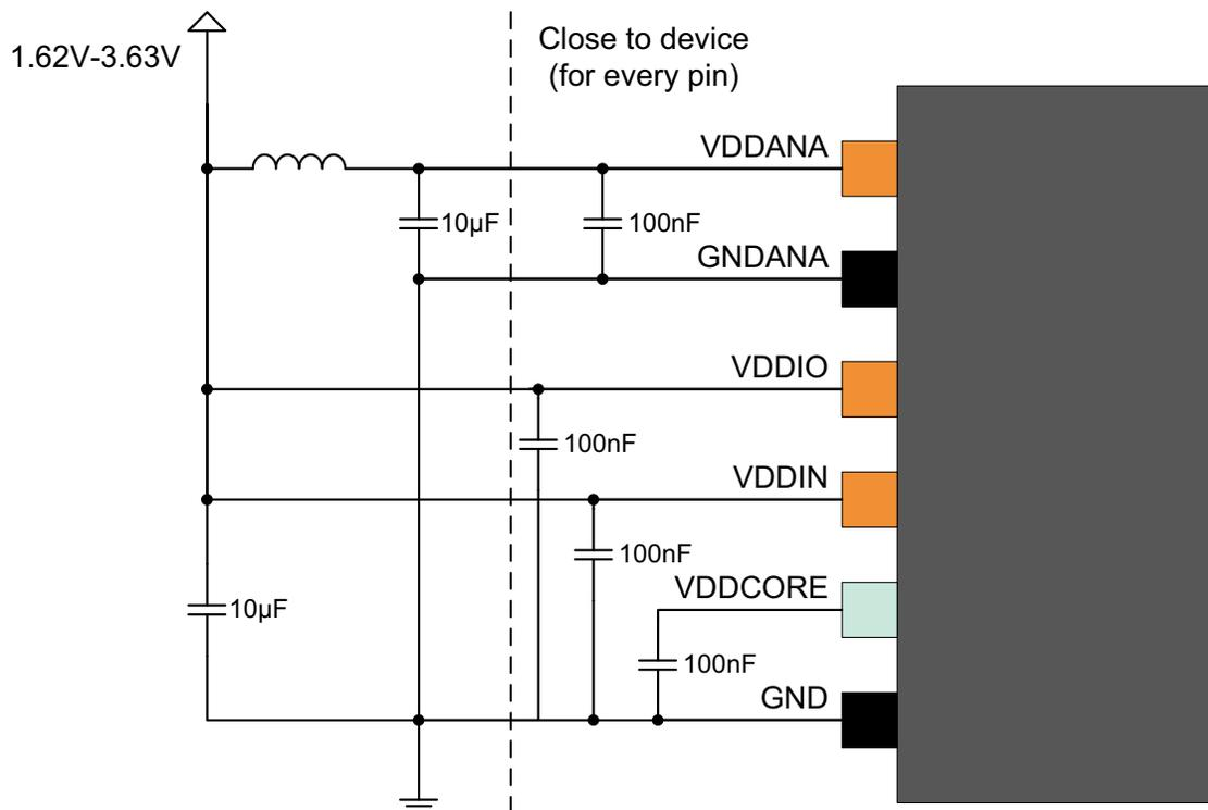
Table 34-1. Power Supply Connections,  $V_{DDCORE}$  From Internal Regulator
