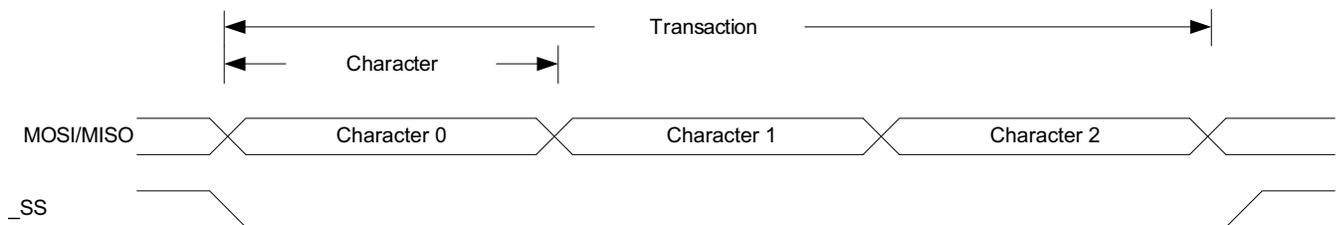
The SPI master must initiate a transaction by pulling low the slave select line (`_SS`) of the desired slave. The master and slave prepare data to be sent in their respective shift registers, and the master generates the serial clock on the SCK line. Data are always shifted from master to slave on the master output, slave input line (MOSI), and from slave to master on the master input, slave output line (MISO). The master signals the end of the transaction by pulling the `_SS` line high.
