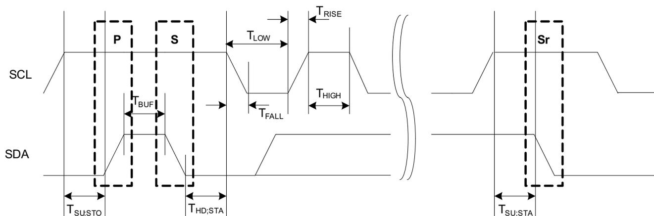
The following parameters are timed using the SCL low time period. This comes from the Master Baud Rate Low bit group in the Baud Rate register (BAUD.BAUDLOW) when non-zero, or the Master Baud Rate bit group in the Baud Rate register (BAUD.BAUD) when BAUD.BAUDLOW is zero.
