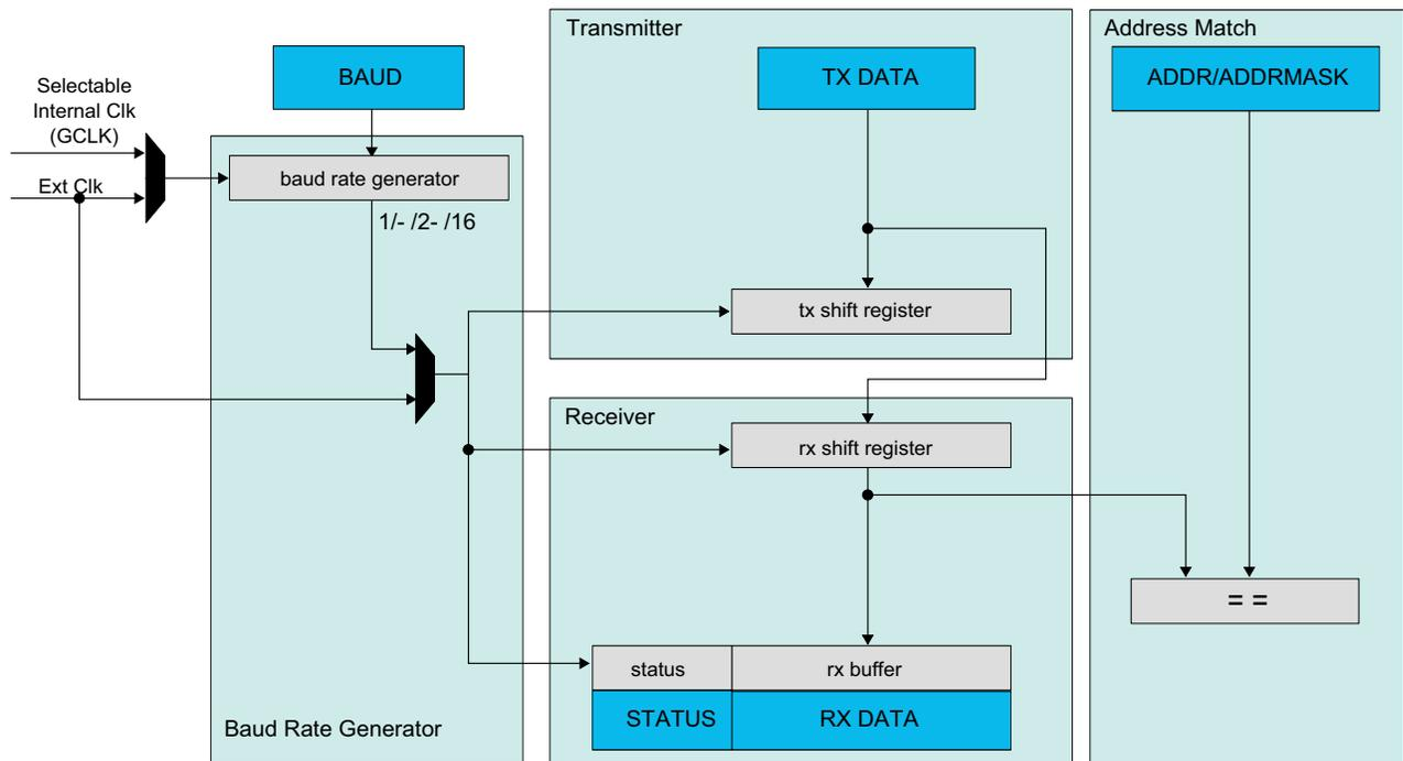
The transmitter consists of a single write buffer and a shift register. The receiver consists of a two-level receive buffer and a shift register. The baud-rate generator is capable of running on the GCLK\_SERCOMx\_CORE clock or an external clock. Address matching logic is included for SPI and I<sup>2</sup>C operation.
