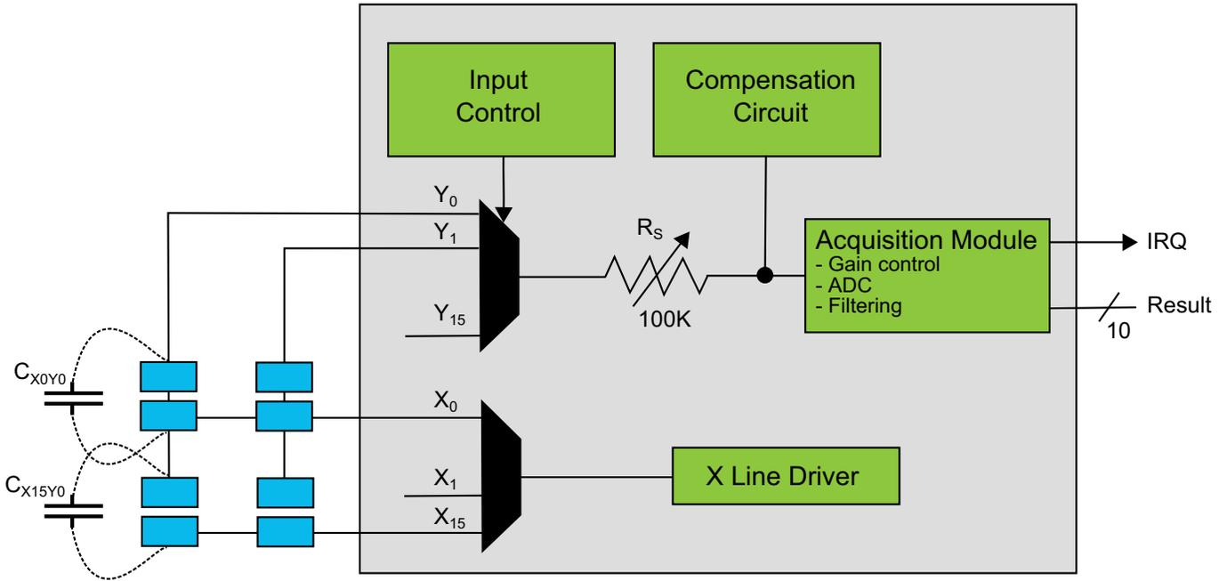
Figure 31-2. PTC Block Diagram Self-capacitance
