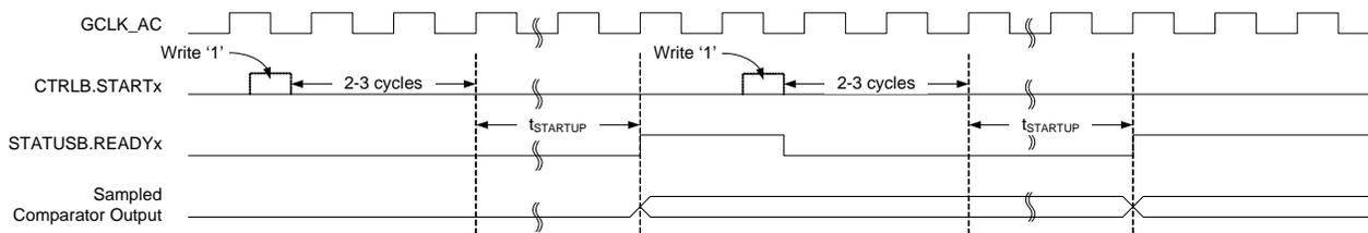
For low-power operation, event-triggered measurements can be performed during sleep modes. When the event occurs, the Power Manager will start GCLK\_AC\_DIG. The comparator is enabled, and after the startup time has passed, a comparison is done and appropriate peripheral events and interrupts are also generated. The comparator and GCLK\_AC\_DIG are then disabled again automatically, unless configured to wake up the system from sleep.
