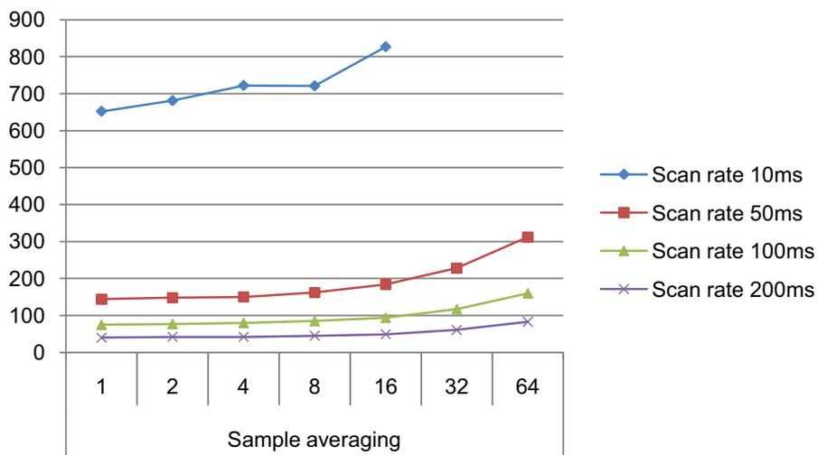
**Figure 32-11. Power consumption [ $\mu$ A].**
