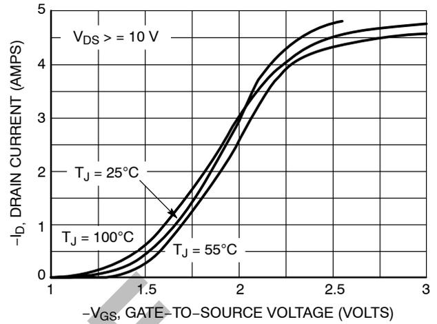
Figure 2. Transfer Characteristics.
