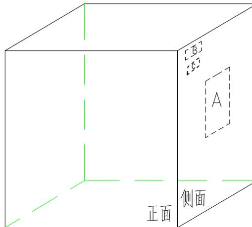
A处:贴LRC标签; B处:贴ROHS标签 C处:贴无卤标签 HF label
