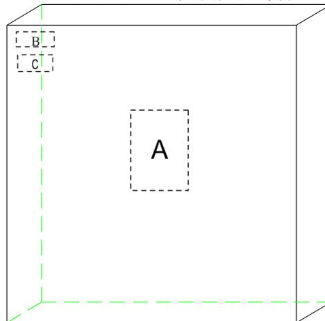
A处:贴LRC标签; B处:贴ROHS标签 C处:贴无卤标签 (无卤产品才贴HF only)
