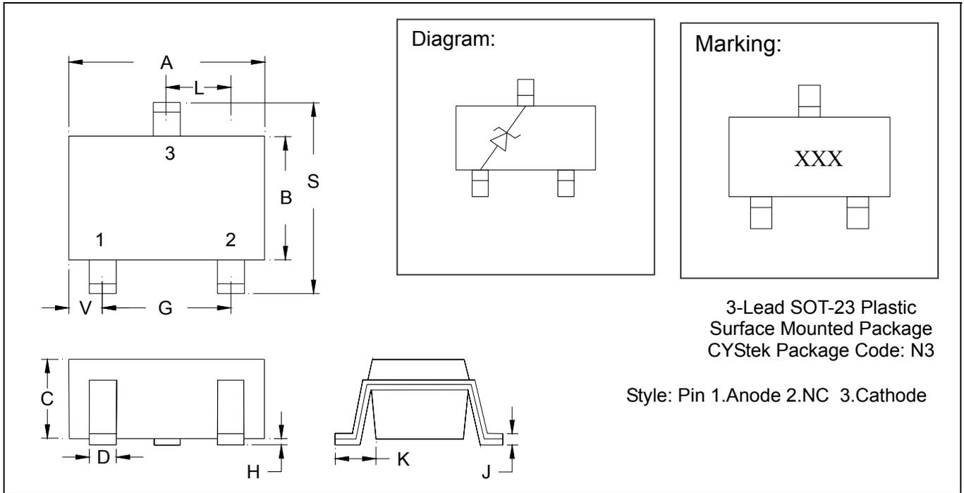
The diagram shows the SOT-23 package with dimensions A through V. It includes a top view with dimensions A, B, C, D, G, H, L, S, V, and a side view with dimensions K and J. A schematic diagram shows the package with a diode symbol. A marking diagram shows the package with 'XXX' marking. The package is a 3-lead SOT-23 Plastic Surface Mounted Package with CYStek Package Code: N3. The style is Pin 1. Anode, Pin 2. NC, Pin 3. Cathode.
