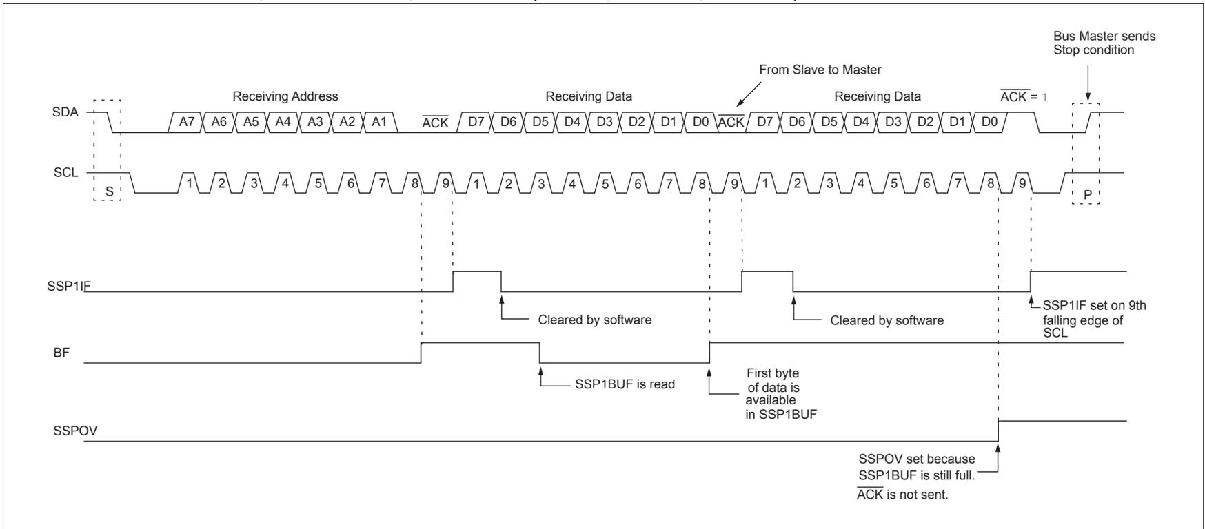
**FIGURE 30-15: I<sup>2</sup>C SLAVE, 7-BIT ADDRESS, RECEPTION (SEN = 1, AHEN = 0, DHEN = 0)**
