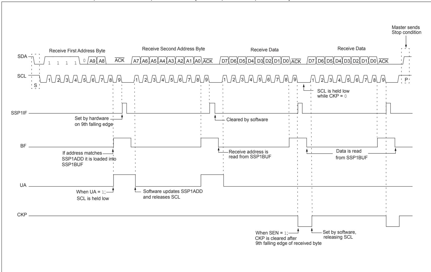
**FIGURE 30-21: I<sup>2</sup>C SLAVE, 10-BIT ADDRESS, RECEPTION (SEN = 0, AHEN = 1, DHEN = 0)**
