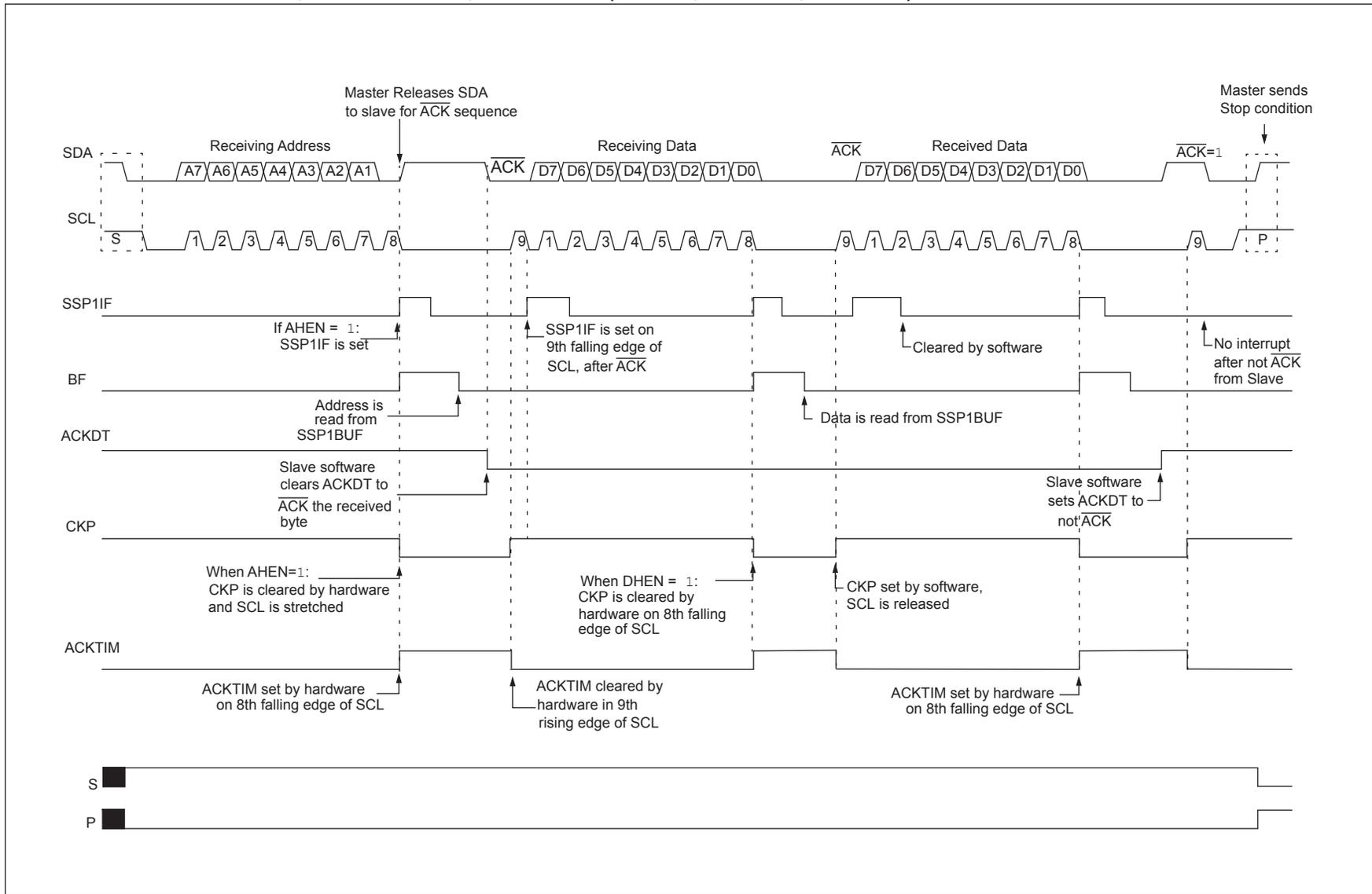
**FIGURE 30-17: I<sup>2</sup>C SLAVE, 7-BIT ADDRESS, RECEPTION (SEN = 1, AHEN = 1, DHEN = 1)**
