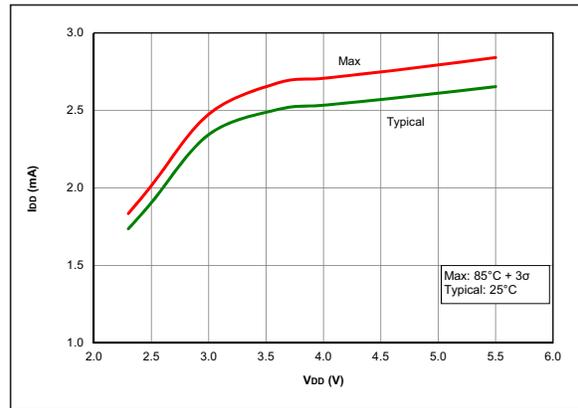
**FIGURE 36-4:**  $I_{DD}$ , HS Oscillator, 32 MHz, PIC16F18324/18344 Only
