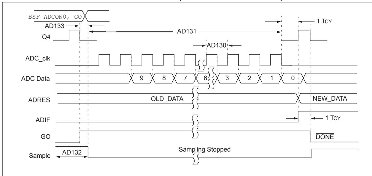
**FIGURE 35-11: ADC CONVERSION TIMING (ADC CLOCK FROM ADCRC)**
