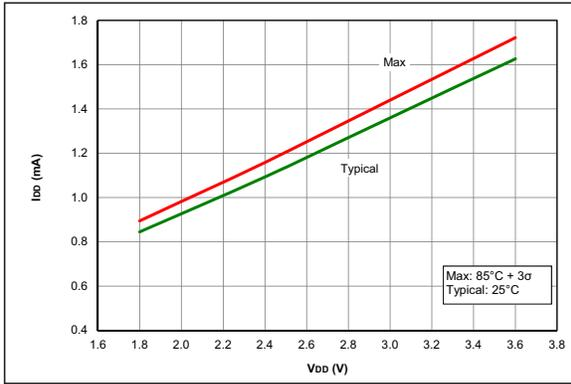
**FIGURE 36-7:**  $I_{DD}$ , HFINTOSC Mode,  $F_{OSC} = 16$  MHz, PIC16LF18324/18344 Only
