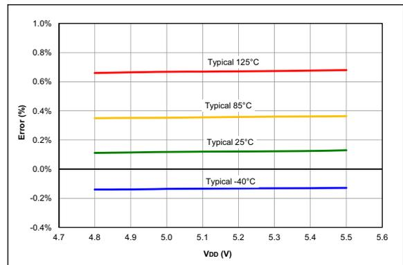
**FIGURE 36-96:** FVR Voltage Error (4x), PIC16F18324/18344 Only
