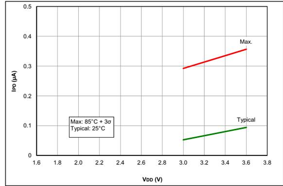
**FIGURE 36-20:** *IPD, Low-Power Brown-out Reset (LPBOR = 0), PIC16LF18324/18344 Only*
