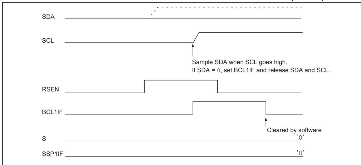
**FIGURE 30-37: BUS COLLISION DURING REPEATED START CONDITION (CASE 2)**
