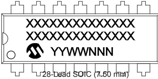
28-Lead SOIC (7.60 mm)
