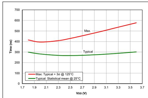
**FIGURE 36-88:** Comparator Response Time Rising edge, PIC16F18324/18344 Only
