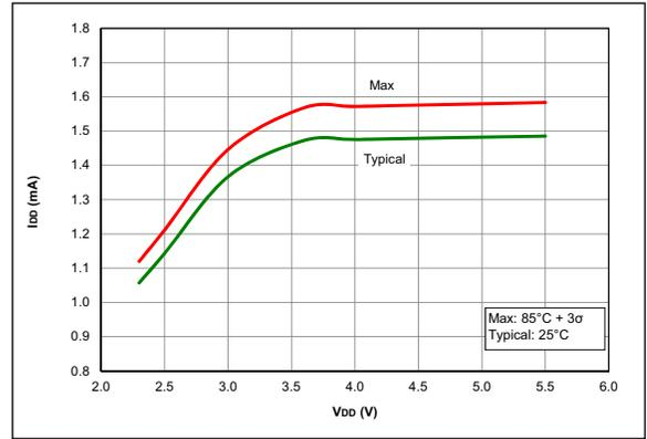
**FIGURE 36-8:**  $I_{DD}$ , HFINTOSC Mode,  $F_{OSC} = 16$  MHz, PIC16F18324/18344 Only
