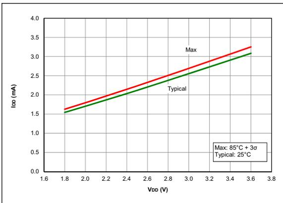
**FIGURE 36-5:**  $I_{DD}$ , HFINTOSC Mode, FOSC = 32 MHz, PIC16LF18324/18344 Only
