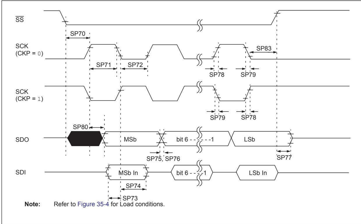
**FIGURE 35-20: SPI SLAVE MODE TIMING (CKE = 1)**
