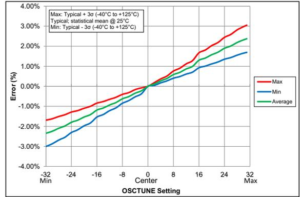
**FIGURE 36-104:** OSCTUNE Center Frequency, PIC16LF18324/18344 Only
