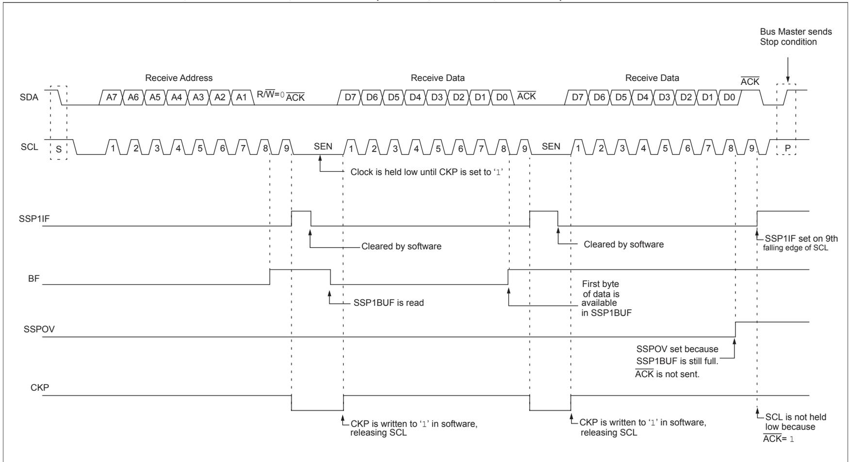
**FIGURE 30-16: I<sup>2</sup>C SLAVE, 7-BIT ADDRESS, RECEPTION (SEN = 0, AHEN = 1, DHEN = 1)**
