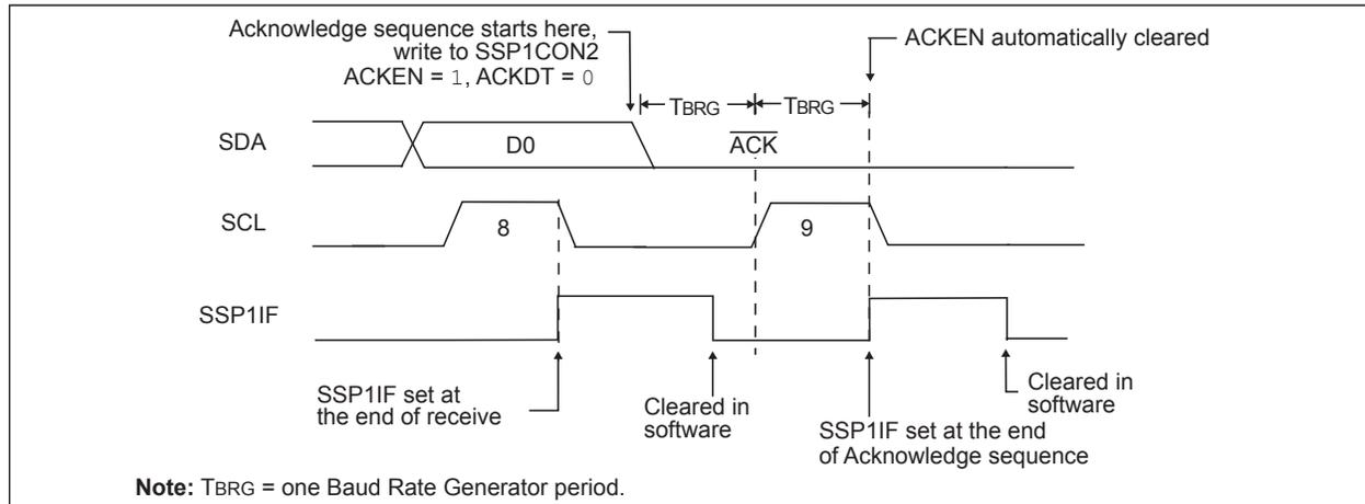
**FIGURE 30-31: STOP CONDITION RECEIVE OR TRANSMIT MODE**
