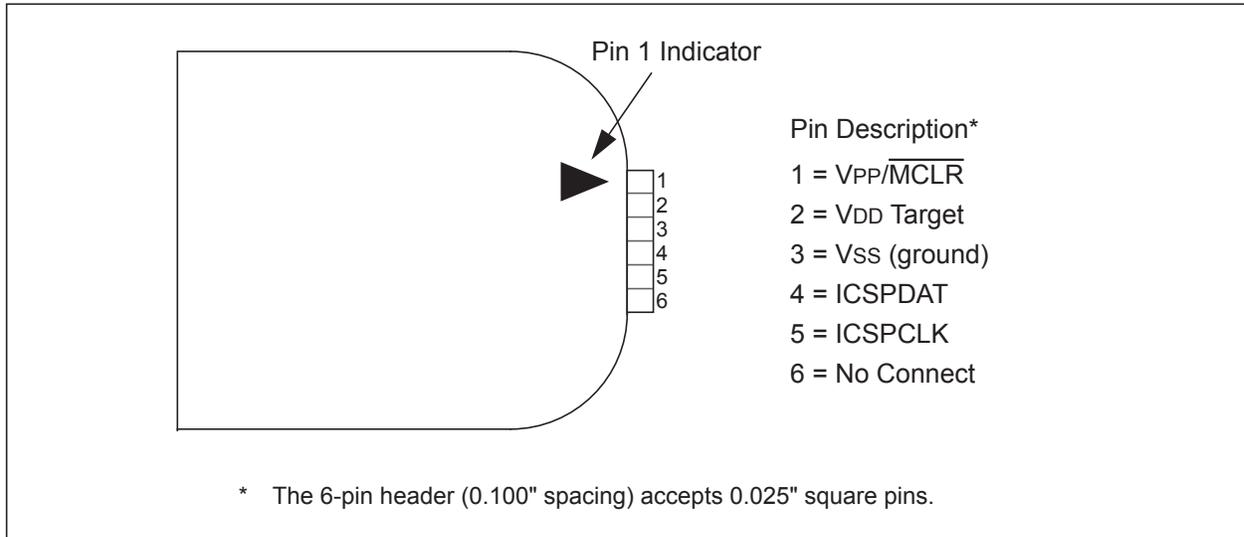
**FIGURE 33-3: TYPICAL CONNECTION FOR ICSP™ PROGRAMMING**
