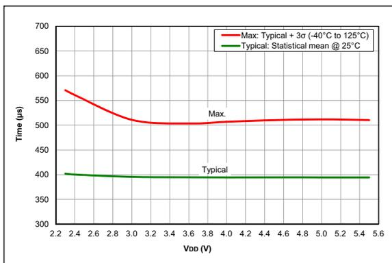
**FIGURE 36-113:** Wake From Sleep, VREGPM = 1, LFINTOSC, PIC16F18324/18344 Only
