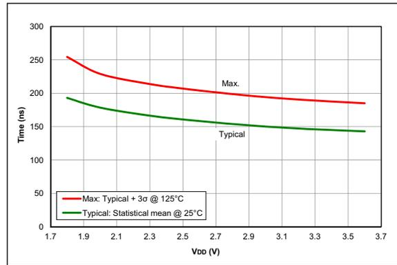
**FIGURE 36-86:** Comparator Response Time Falling edge, PIC16LF18324/18344 Only
