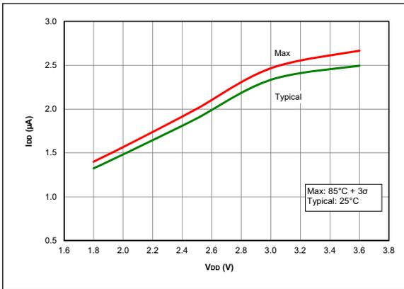
**FIGURE 36-3:**  $I_{DD}$ , HS Oscillator, 32 MHz, PIC16LF18324/18344 Only
