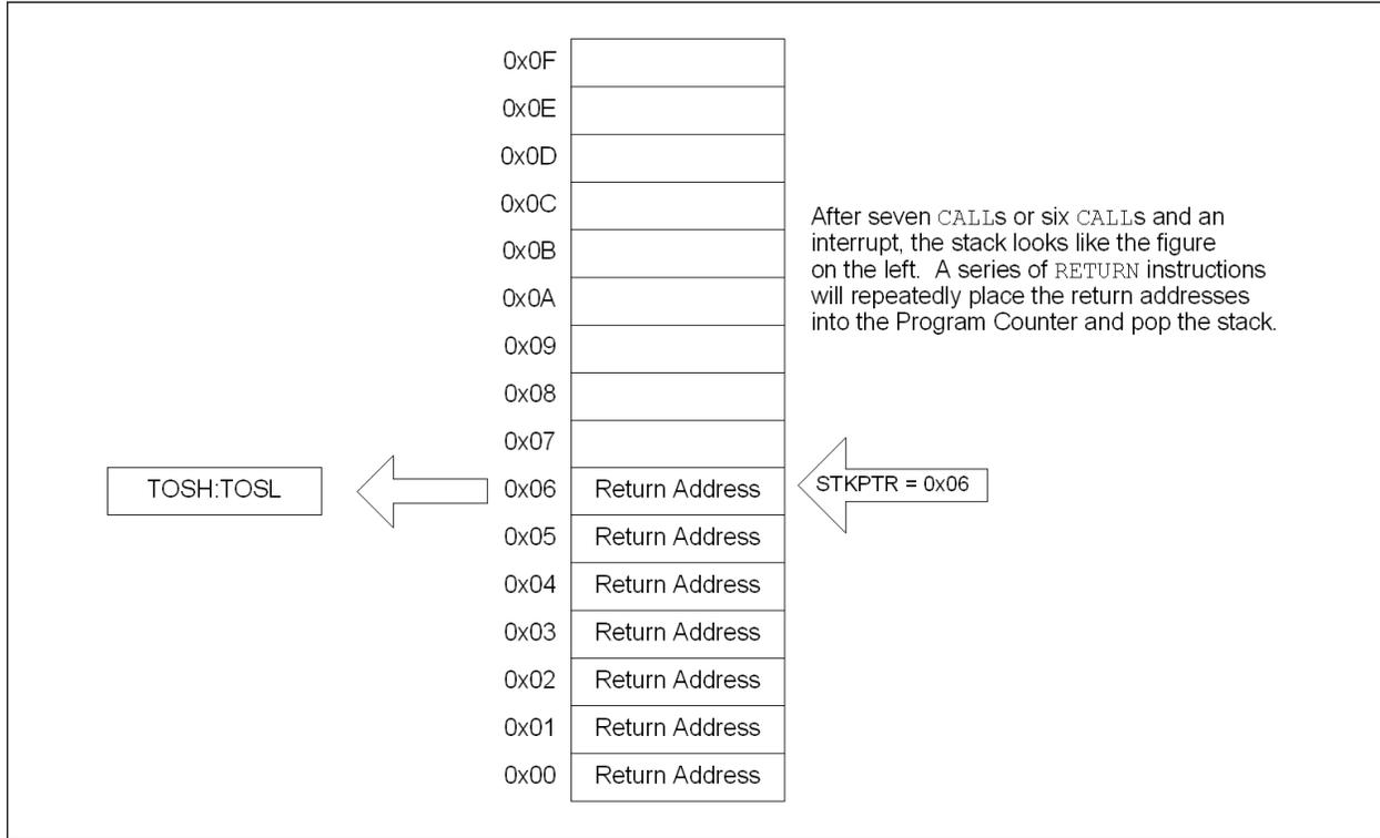
**FIGURE 4-7: ACCESSING THE STACK EXAMPLE 4**
