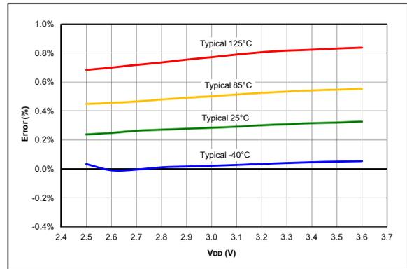
**FIGURE 36-94:** FVR Voltage Error (2x), PIC16LF18324/18344 Only
