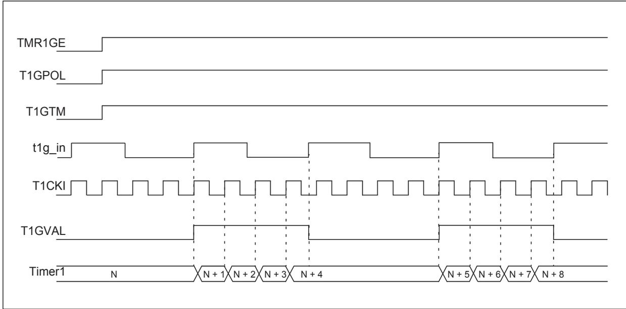
**FIGURE 27-5: TIMER1 GATE SINGLE-PULSE MODE**
