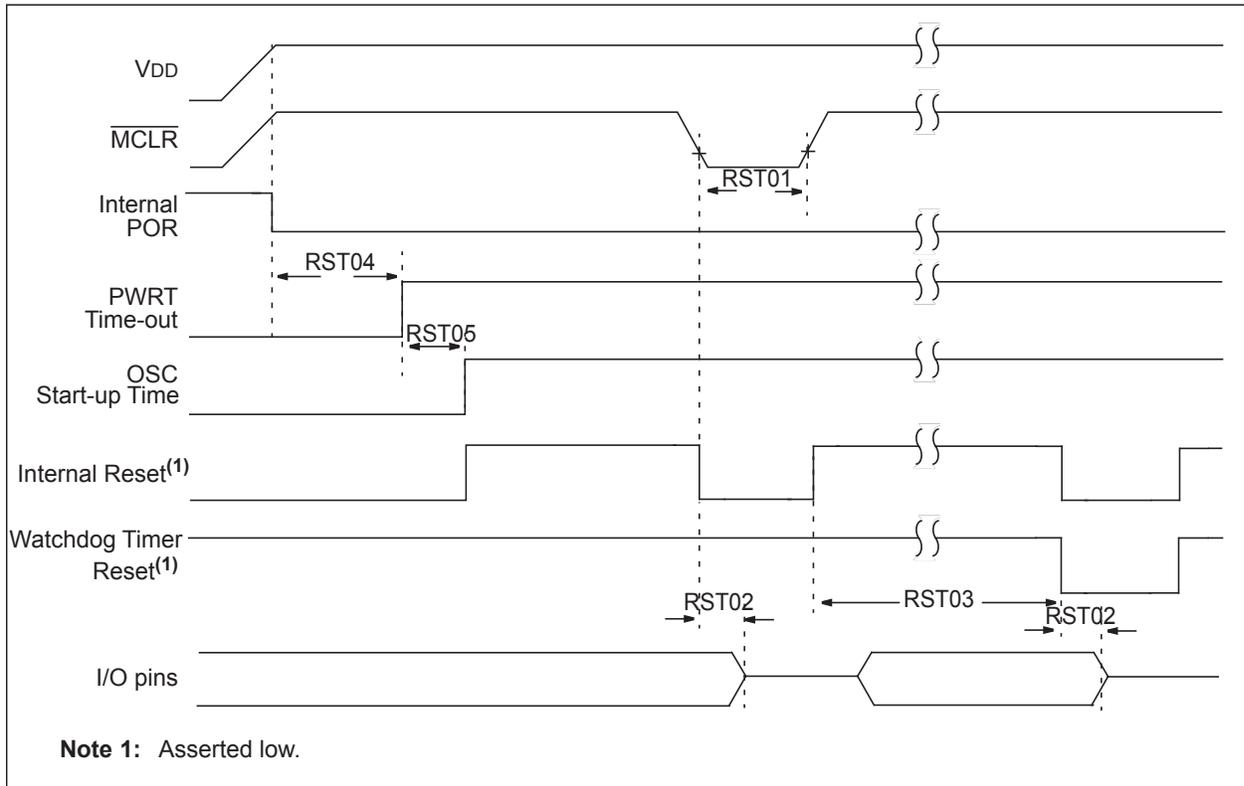
**FIGURE 35-9: BROWN-OUT RESET TIMING AND CHARACTERISTICS**
