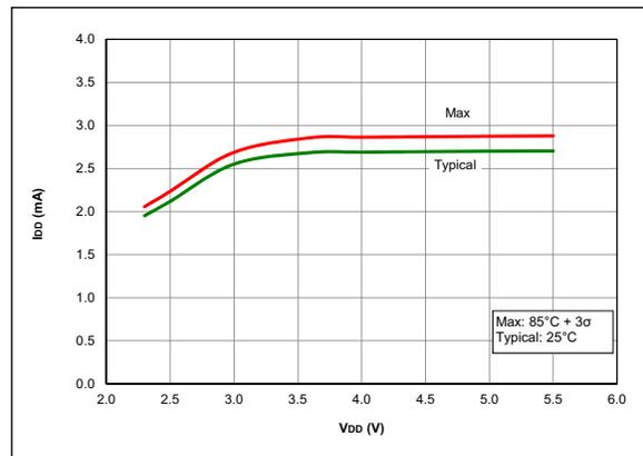
**FIGURE 36-6:**  $I_{DD}$ , HFINTOSC Mode, FOSC = 32 MHz, PIC16F18324/18344 Only
