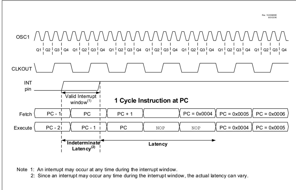
**FIGURE 8-3: INT PIN INTERRUPT TIMING**
