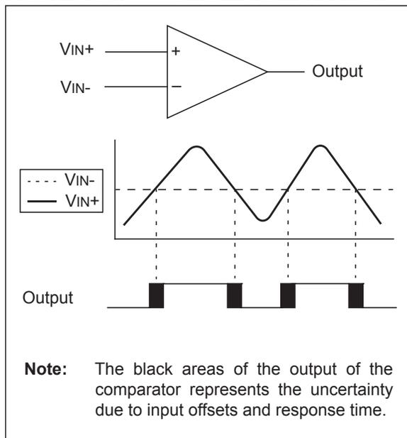
**FIGURE 18-2: COMPARATOR MODULE SIMPLIFIED BLOCK DIAGRAM**
