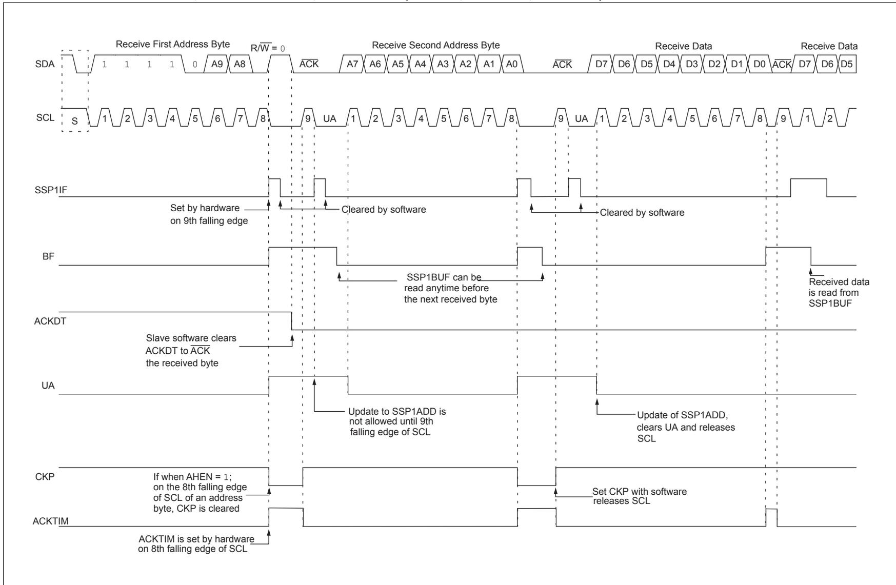
**FIGURE 30-22: I<sup>2</sup>C SLAVE, 10-BIT ADDRESS, TRANSMISSION (SEN = 0, AHEN = 0, DHEN = 0)**
