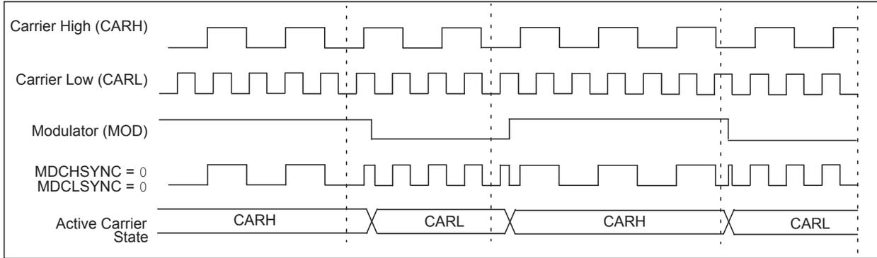
**FIGURE 25-4: CARRIER HIGH SYNCHRONIZATION (MDSHSYNC = 1, MDCLSYNC = 0)**
