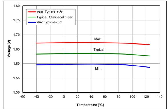
**FIGURE 36-106:** POR Rearm Voltage, Normal Power Mode, PIC16F18324/18344 Only
