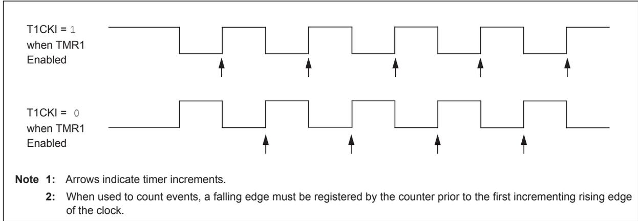
**FIGURE 27-3: TIMER1 GATE ENABLE MODE**
