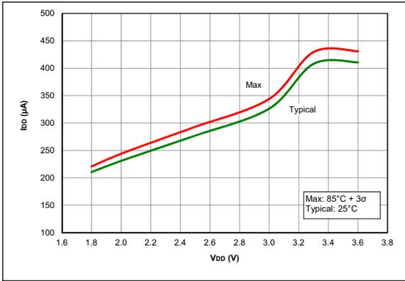
**FIGURE 36-1:**  $I_{DD}$ , XT Oscillator, 4 MHz, PIC16LF18324/18344 Only
