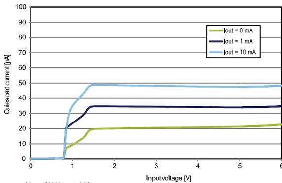
$V_{IN} = 2 \text{ V}, V_{OUT} = 1 \text{ V}$
