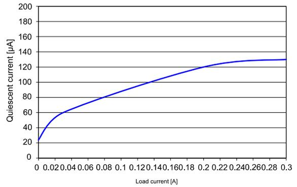
$V_{IN} = 2.8 \text{ V}, V_{OUT} = 1.8 \text{ V}, I_O = 0 \text{ to } 0.3 \text{ A}$
