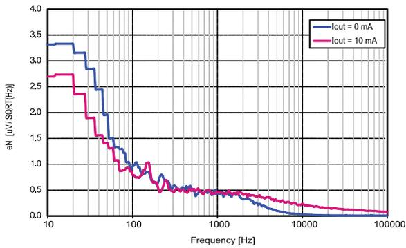
$V_{IN} = 2.0\text{ V}$ ,  $V_{OUT} = 1.0\text{ V}$ ,  $C_{IN} = C_{OUT} = 1\text{ }\mu\text{F}$
