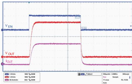
$V_{IN} = 5.5\text{ V}$ ,  $V_{EN} = 0\text{ V to } 2\text{ V}$ ,  $I_{OUT} = 0.2\text{ A}$ ,  $V_{OUT} = 5\text{ V}$ ,  $T_r = 5\text{ }\mu\text{s}$
