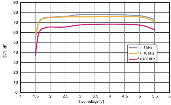
$I_{OUT} = 30\text{ mA}$ ,  $V_{OUT} = 1\text{ V}$ ,  $C_{OUT} = 1\text{ }\mu\text{F}$
