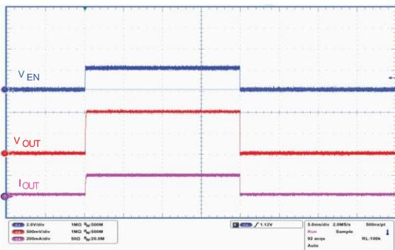
$V_{IN} = 2\text{ V}$ ,  $V_{EN} = 0\text{ V to } 2\text{ V}$ ,  $I_{OUT} = 0.2\text{ A}$ ,  $V_{OUT} = 1\text{ V}$ ,  $T_r = 5\text{ }\mu\text{s}$
