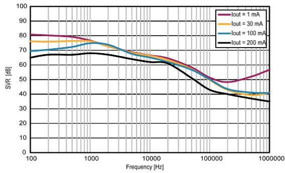
$V_{IN} = 2\text{ V} \pm 200\text{ mV}$ ,  $V_{OUT} = 1\text{ V}$ ,  $C_{OUT} = 1\text{ }\mu\text{F}$
