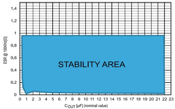
$V_{IN}$  from 2 to 5.5 V,  $I_{OUT}$  from 0 to 300 mA,  $C_{IN} = 1\text{ }\mu\text{F}$
