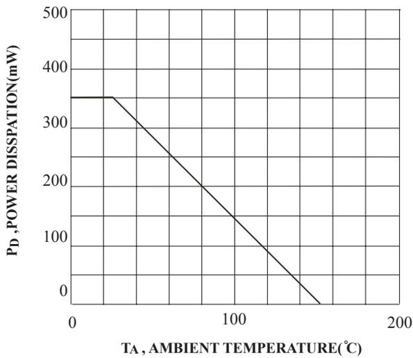
**FIG.1 Power Derating Curve, total package**
